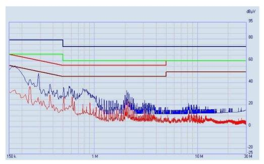
图 15. Conducted Emission Plot for ISOW7841-Based BIM
