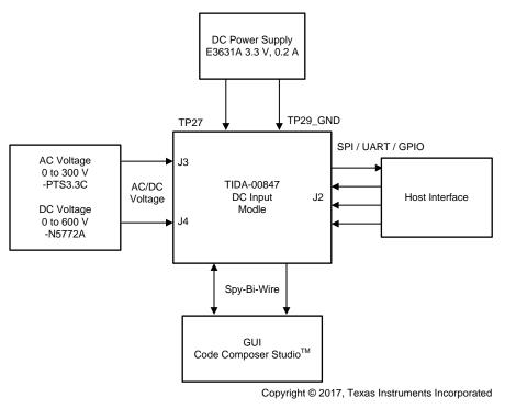
图 9. Test Setup for AC/DC BIM Performance Testing
