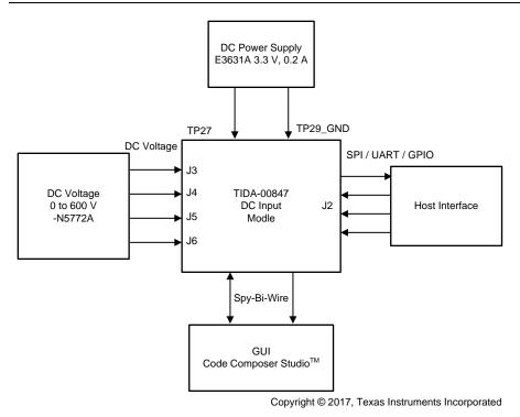
图 10. Test Setup DC BIM Performance Testing
