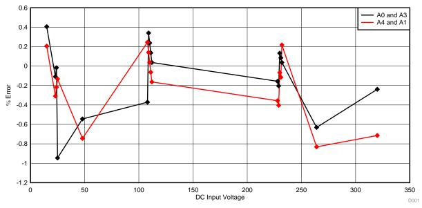
图 14. DC Input Voltage versus % Error of Measured Value Plot
