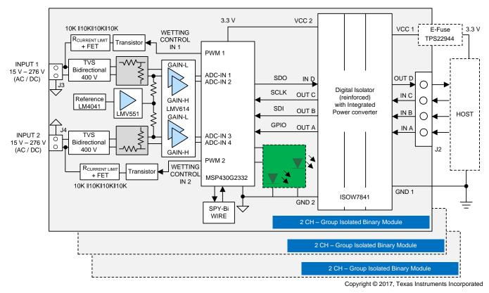
图 3. AC/DC BIM With ISOW7841 Integrated Power Converter
