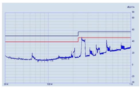
图 16. Radiated Emission Plot for ISOW7841-Based BIM at 3 m
