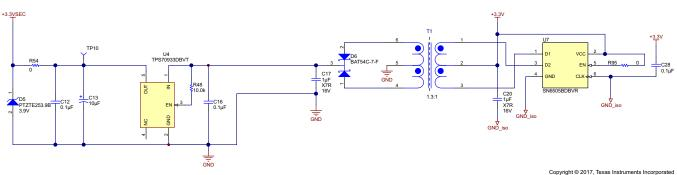
图 7. Transformer Driver-Based Isolated Power for Digital Isolator Interface
