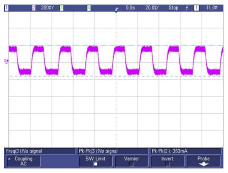
图 12. Input Switching Current for 75-mA Output Loading
