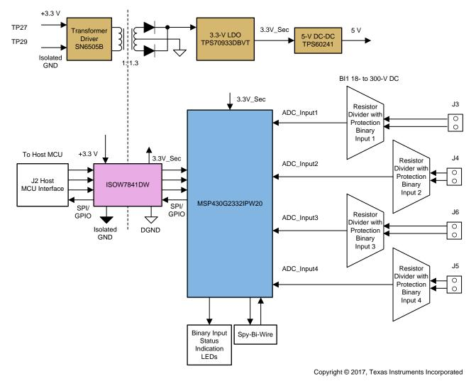
图 2. Four-Channel DC BIM With MSP430G2332 and ISO7741 With Transformer Driver
