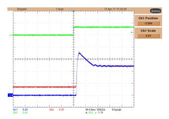
图 71. 12-V Circuit Breaker Turnon to 12-V Terminal (Blue = KL30-31 Terminal, Green = UVLO, and Red = P12V)
