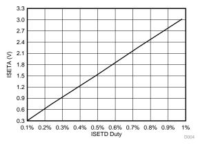
图 74. Relationship Between ISETD Duty Cycle and ISETA Voltage: C912 = 3.3 nF, f<sub>ISED</sub> = 48.8 kHz
