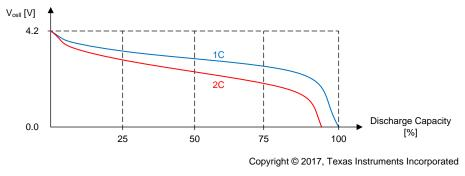
图 2. Li-Pol Cell Typical Discharge Curve
