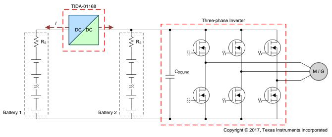
图 1. Dual Battery System Combined With Motor Generator
