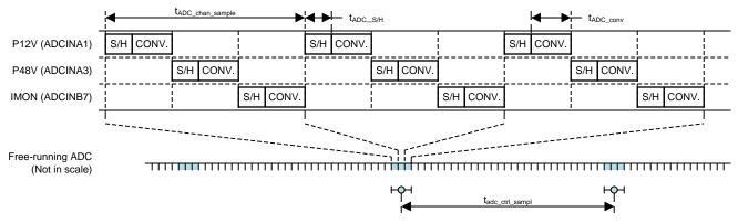
图 38. ADC Channels Conversion Timing Diagram
