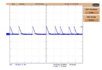
图 82. MC33063A-Q1 Pre-Boost Converter Output Ripple at 50 mA
