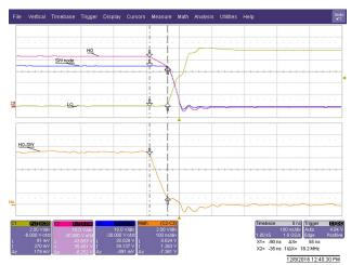
图 69. Switching Waveforms With Fixed Dead-Time Settings (R906 = 10 k) – Detail
