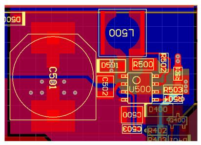
图 31. Bias Supplies PCB Layout—MC33063A-Q1 Pre-Boost Converter
