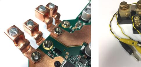
图 51. Modified Terminals for TIDA-01168
