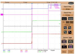
图 81. External Watchdog Behavior During Start-Up: (Blue = nRST, Violet = NSHDN, Green = P10V, and Red = P3V#)
