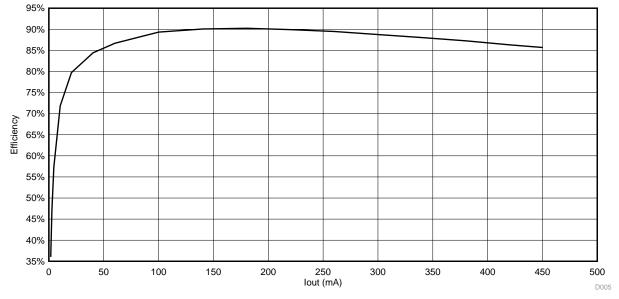
图 92. Efficiency Plot for TPS560200-Q1 Step-Down Converter V<sub>IN</sub> = 10 V, V<sub>OUT</sub> = 3.3 V
