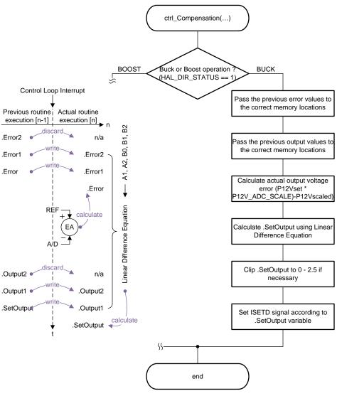
图 47. Digital Compensator Flow Chart
