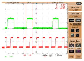
图 78. I <sup>2</sup> C Bus TMP102-Q1 Single Frame Timing (Detail)
