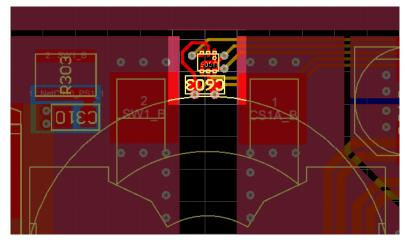
图 28. Diag PCB Layout—TMP102-Q1 Temperature Sensor in Power Stage
