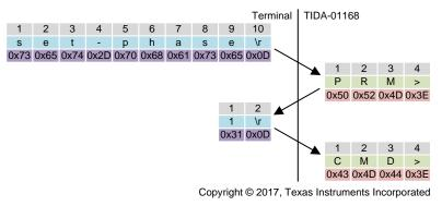
图 62. Example of Serial Communication Between Terminal and TIDA-01168
