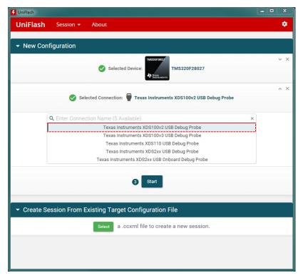
图 56. Uniflash V4—Selecting Communication Interface
