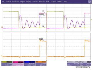
图 67. Switching Waveforms With Adaptive Dead-Time Settings (Detail)
