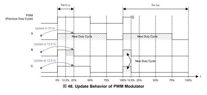
注: The selected C2000 MCUs from Texas Instruments have an enhanced pulse-width modulator (ePWM) module with a high-resolution pulse-width modulator (HRPWM) extension. The HRPWM module extends the time resolution capabilities of the conventionally-derived digital pulse-width modulator (ePWM). HRPWM is typically used when the PWM resolution falls approximately below 9 to 10 bits.
