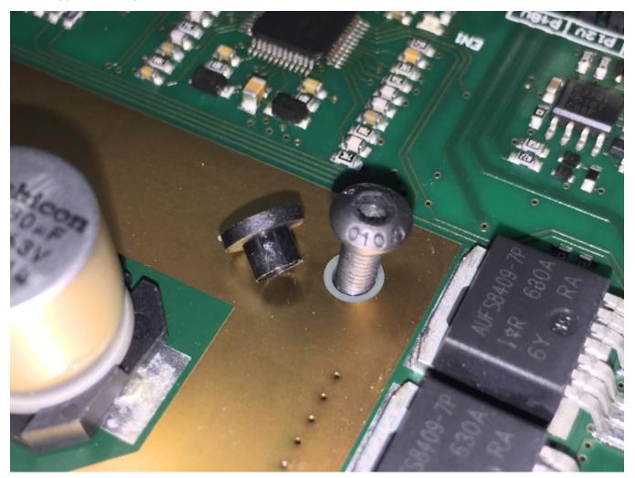
图 94. Hole for M3 Screw and Isolation Spacer
