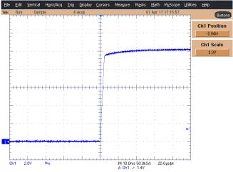
图 87. LM5010A-Q1 Step-Down Converter Start-Up Behavior to 200-Ω Load
