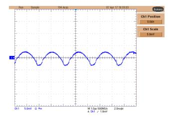
图 83. LM5010A-Q1 Step-Down Converter Output Ripple in CCM Mode
