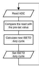
图 35. Simplified Control-Loop Flow Chart
