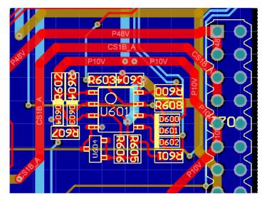
图 27. Diag PCB Layout—External Watchdog and Voltage Supervisor
