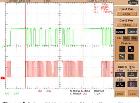
图 77. I <sup>2</sup> C Bus TMP102-Q1 Single Frame Timing
