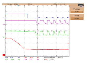
图 80. External Watchdog Behavior During Shutdown: (Blue = nRST, Violet = P3V3, Green = P10V, and Red = VIN\_LM)
