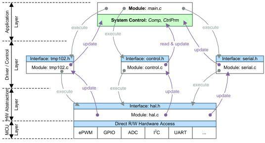
图 33. Software Architecture Diagram for TIDA-01168
