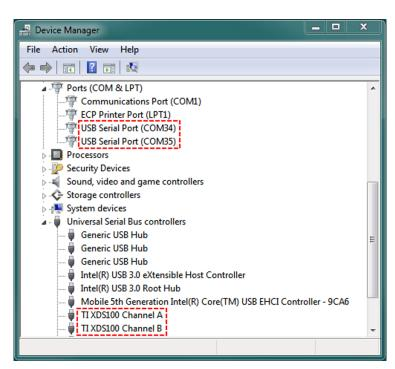
图 53. Properly Installed and Configured XDS100V2 Driver
