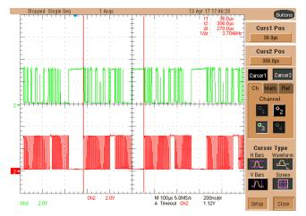
图 76. I<sup>2</sup>C Bus TMP102-Q1 Frames Timing
