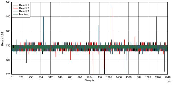
图 39. Effect of Median Filter in Time Domain
