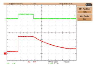
图 72. 12-V Circuit Breaker Turnoff From 12-V Terminal (Green = UVLO, Red = P12V)
