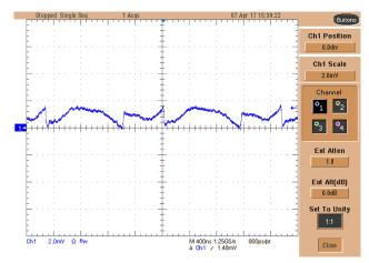
Note the effect of ESL of the output capacitors and the very fine oscilloscope vertical amplifier settings.
