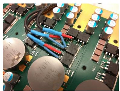
图 64. Measurement Technique for Switching Node and Gate Signals Using DIY 1:21 Passive Probe[27].
