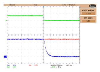
图 73. 12-V Circuit Breaker Turnoff to 12-V Terminal (Blue = KL30-31 Terminal, Green = UVLO, and Red = P12V)
