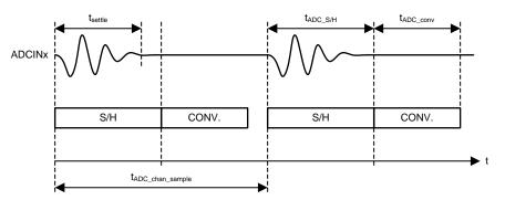
图 42. Sample-and-Hold Circuit Timing
