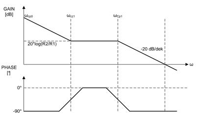
图 44. Phase and Gain of Type-II Compensator
