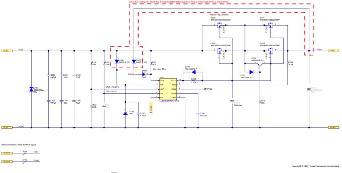
图 14 shows a schematic of the 48-V circuit breaker implementation.
