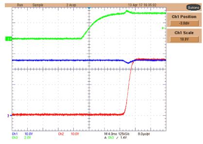
图 63. 48-V Circuit Breaker Turnon from KL40-41 Terminal (Blue = KL40-41 Terminal, Green = EN48, and Red = P48V)
