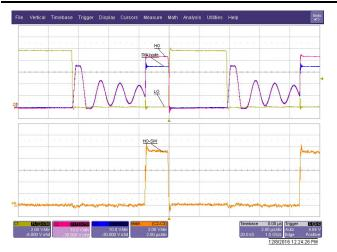
图 65. Switching Waveforms With Adaptive Dead-Time Settings
