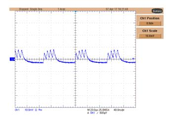
图 85. TPS560200-Q1 Step-Down Converter Output Ripple at 10-mA Light-Load Operation
