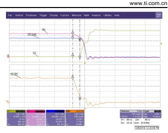
图 66. Switching Waveforms With Adaptive Dead-Time Settings (Detail)
