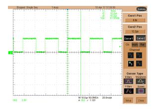
图 75. Timing of Control loop ISR Measured on Testpin ADCINB2 (D700)
