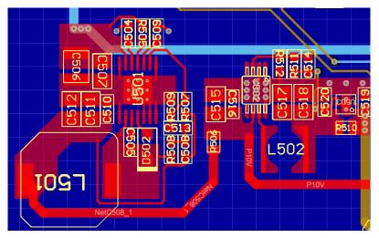
图 30. Bias Supplies PCB Layout—LM5010-Q1 and TPS560200-Q1 Step-Down Converters
