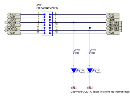
图 32. System Interface Schematic
