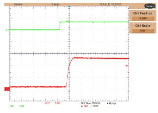
图 70. 12-V Circuit Breaker Turnon From 12-V Terminal (Green = UVLO, Red = P12V)
