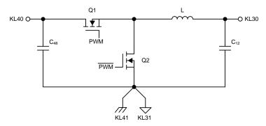
图 6. Non-Isolated Synchronous Step-Down Converter
