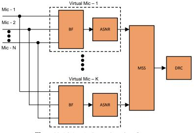
图 11. Multi-Angle Beamforming System
