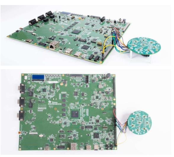
图 5. EVMK2G With CMB Connected
