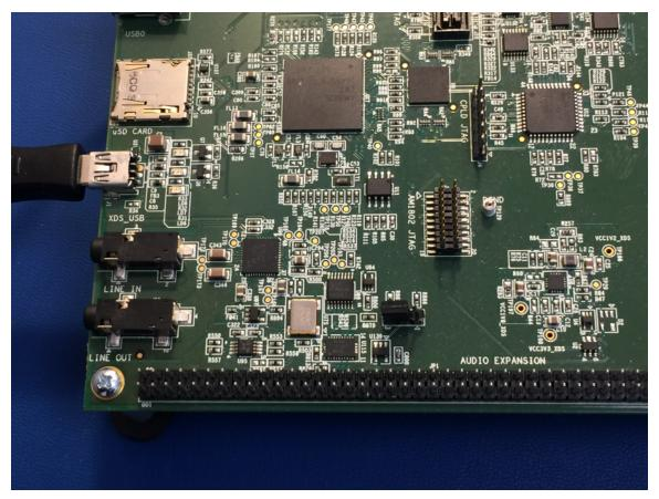
图 6. Audio Extension and Audio Line Out on EVMK2G
