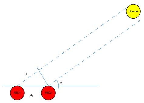
图 9. Differences in Distance, Time, and Phase Between Two Microphones
