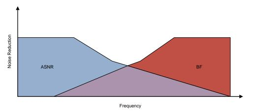
图 10. ASNR and BF Noise Reduction as a Function of Noise Frequency
