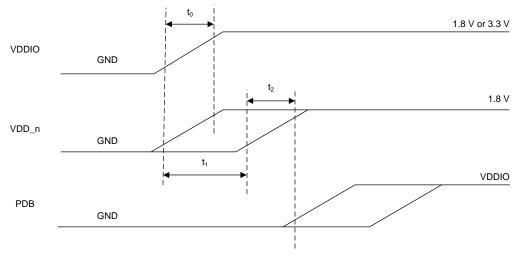
图 10. Target Power-up Sequence
