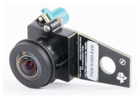
图 11. TIDA-01003 Completed Assembly
