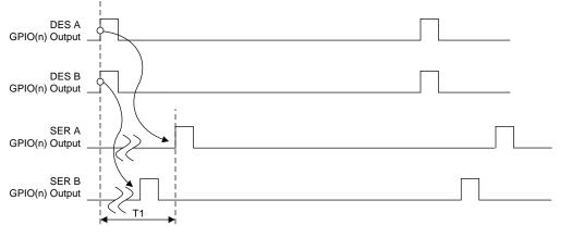
图 9. GPIO Maximum Latency
