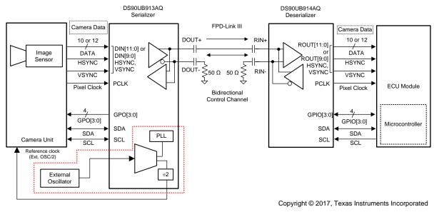
图 7. Typical Operation in External Oscillator Mode
