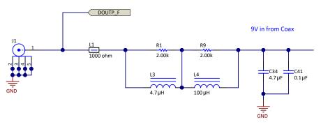
图 6. Power Over Coax Schematic
