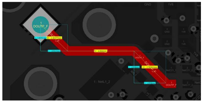
图 31. High-Speed Data Line Trace
