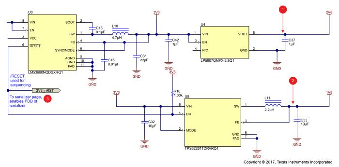
图 13. Power-up Sequence for Test Lead Connections
