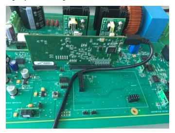
图 18. USB Connection on Board
