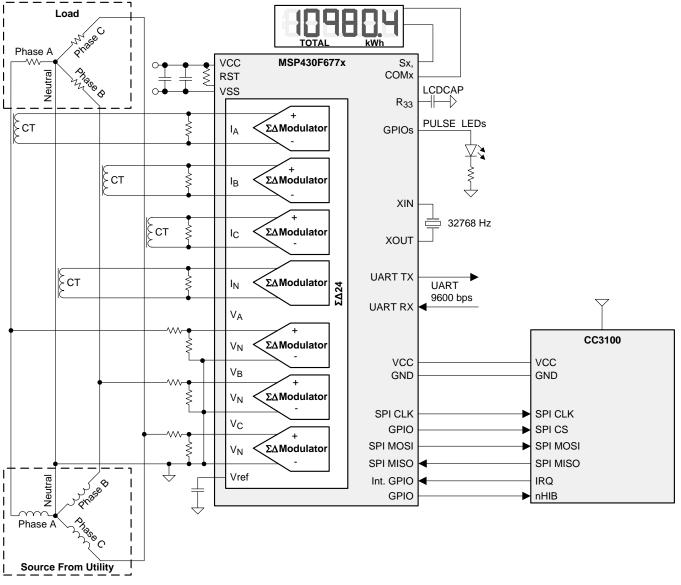
图 29. TIDC-3PHMTR-WIFIXR System Block Diagram
