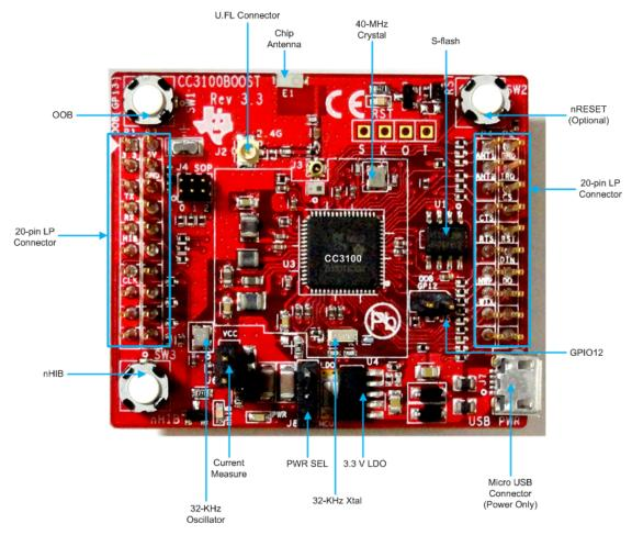
图 14. Front View of CC3100BOOST With Highlighted Components
