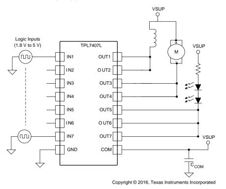
图 8. TPL707L Sample Application Schematic
