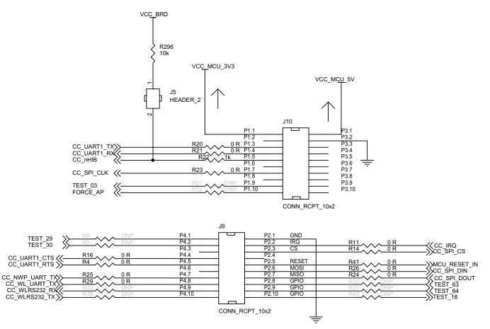
图 22. Connections on CC3100BOOST BoosterPack Female Connectors
