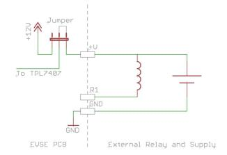
图 16. Relay With External Supply
