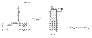
图 20. Connections on CC3100\_EM\_BP\_ADAPTER EM Female Connectors
