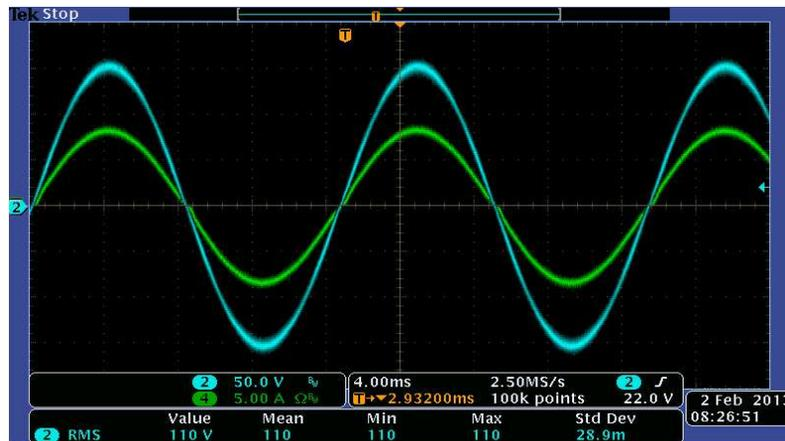
图 14. IL PFC Input Voltage and Current at 550W Load and 110Vrms Input
