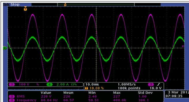
Ch3 -Vin, Ch4-Iin, Vrms=230V, Vbus=390V, Pout=375W
