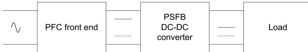
**图 2. Isolated AC-DC Rectifier Block Diagram**
