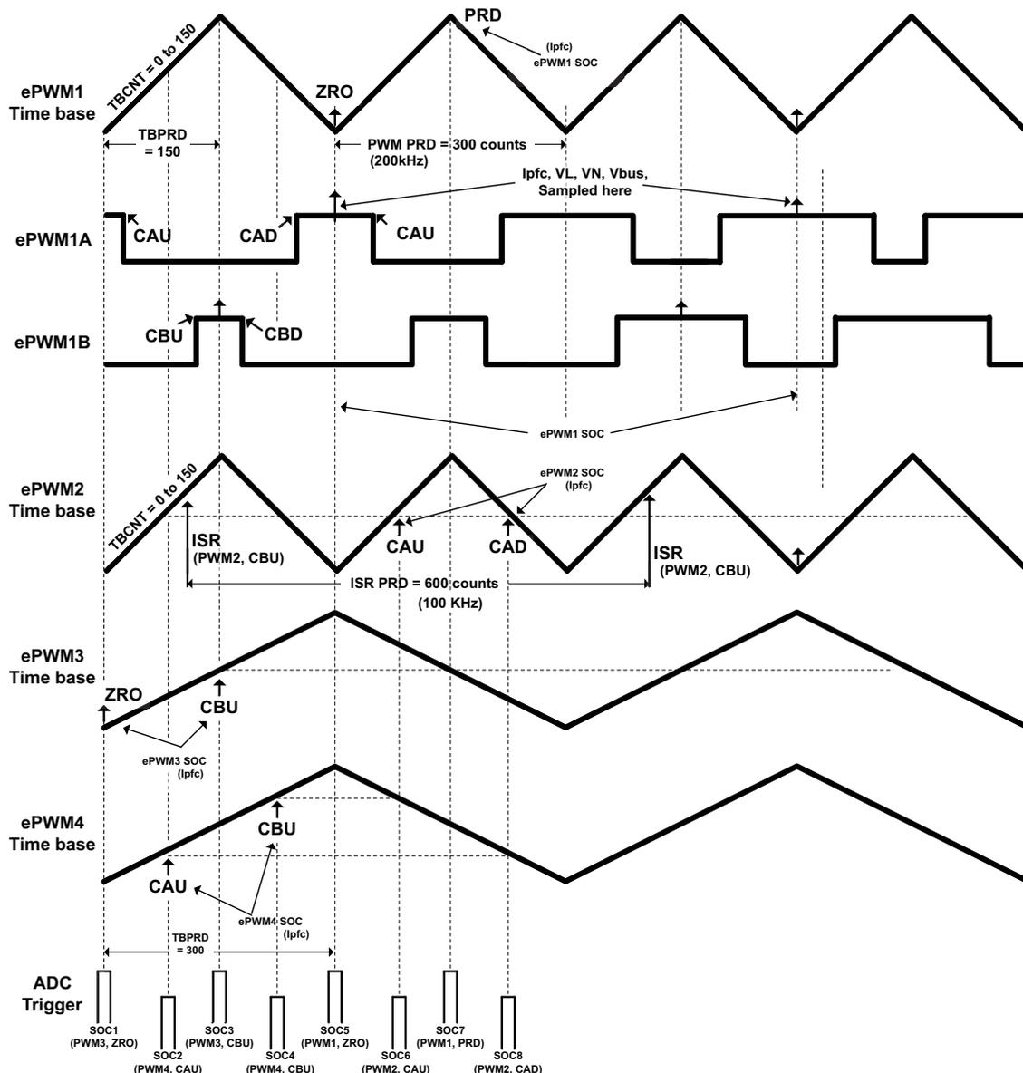
图 8. PWM generation and ADC Sampling
