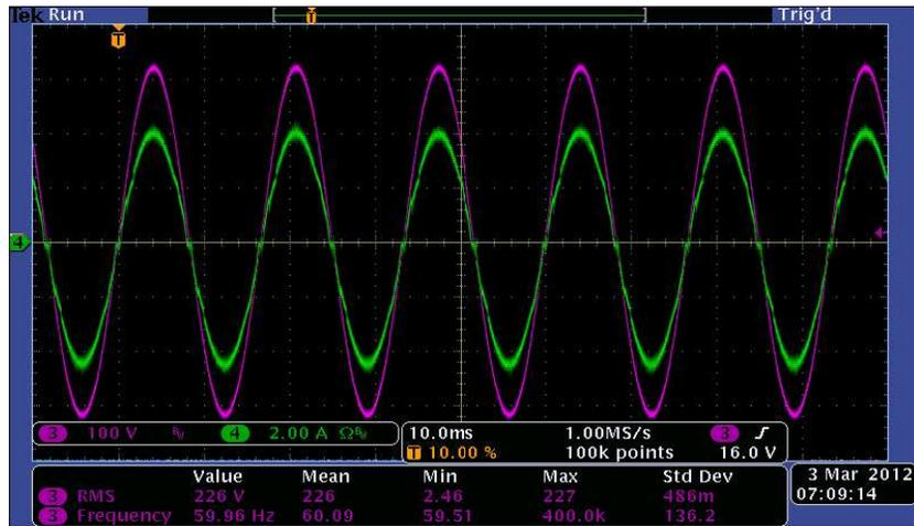
(1) Ch3 -Vin, Ch4-Iin, Vrms=230V, Vbus=390V, Pout=700W
