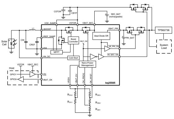
图 3. bq25505 Functional Block Diagram
