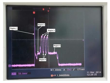
图 14. Power Drawn During Beacon Transmission
