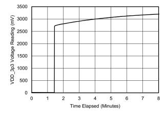
图 24. VDD\_3p3 After Load Switch as Controlled by bq25505
