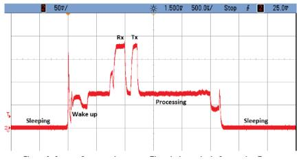
图 7. Current Consumption versus Time During a Single Connection Event
