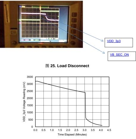
图 26. VDD\_3p3 After Load Switch as Controlled by bq25505
