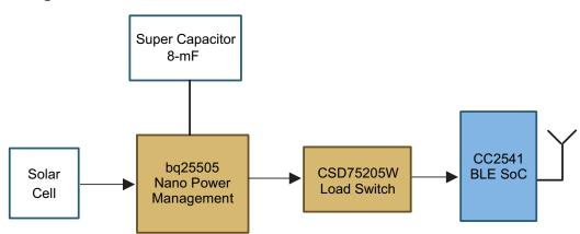
图 2. Bluetooth Low Energy Beacon Subsystem Block Diagram
