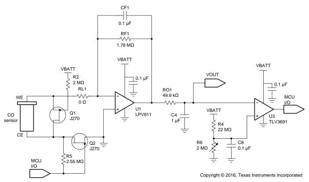
图 9. CO Sensor Analog Signal Path Schematic
