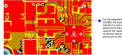
For the integrated DC-DC converter in the CC2650, the input capacitors C33 and C34, inductor L4, and output capacitor C37 were placed such that a common ground area is used for the capacitors. The ground area had no ground vias and was directly connected the ground pin on the CC2650.
