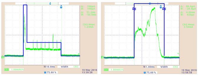
图 11. Power Profile During Startup Period
