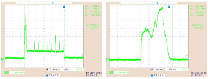
图 29. Startup Current at Beginning of Test State
