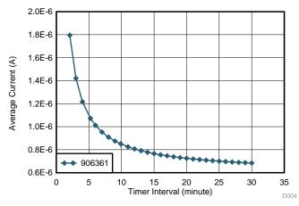
图 33. Combined Standby and Test State Average Current versus Timer Interval
