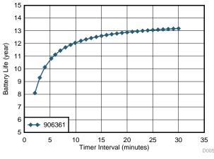
图 34. Battery Life versus Timer Interval
