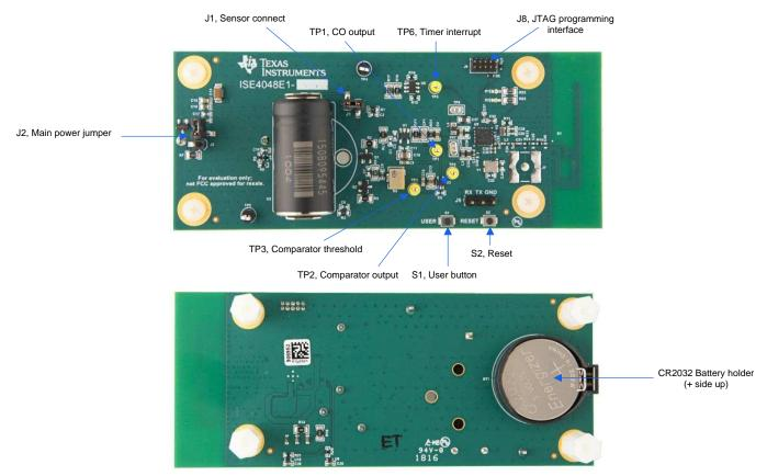
图 16. Low-Power Carbon Monoxide Sensor Reference Design Hardware Description
