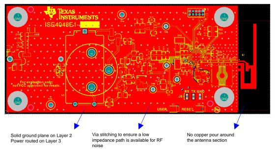
图 40. Low-Power Carbon Monoxide Sensor Reference Design Layout Guidelines
