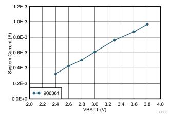
图 32. Alarm State Current Consumption Across System Voltage
