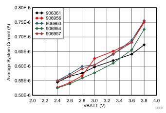
图 28. Standby State Current Consumption Across System Voltage
