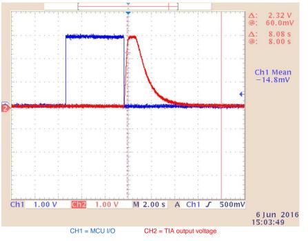
图 5. Normal Sensor Response to Test Current
