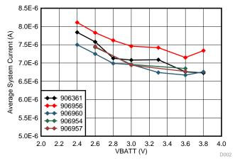
图 31. Pre-Alarm State Current Consumption Across System Voltage
