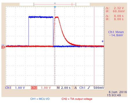
图 6. Normal Sensor Response to Test Current (With CO Gas)
