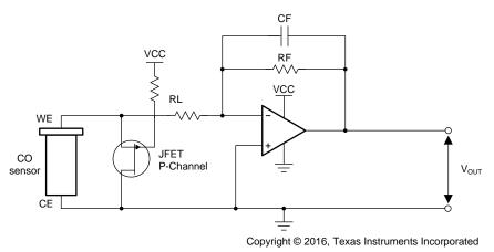
图 4. Sensor Anti-Polarization Technique Using P-Channel JFET
