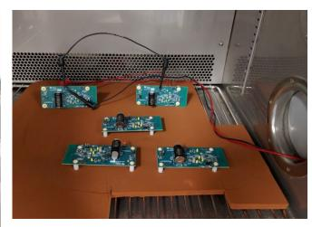
图 27. Reference Design PCBs Inside Environmental Chamber
