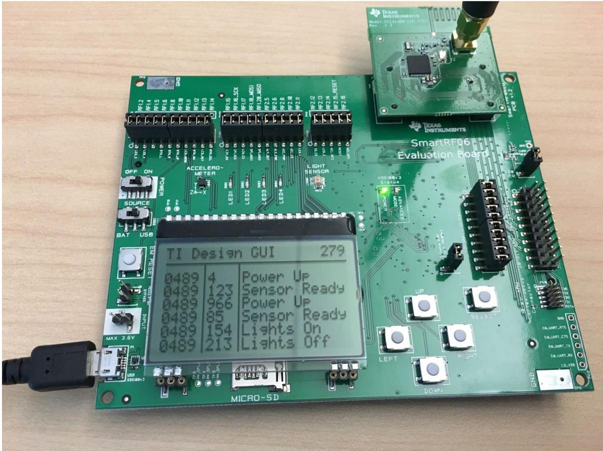
图 12. Building Automation Sub-1GHz Sniffer GUI
