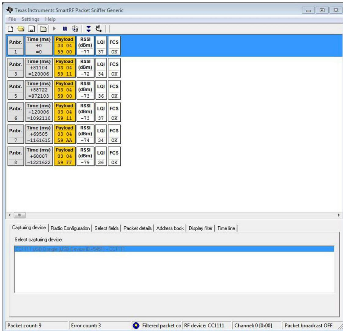
图 16. Packet Sniffer Software, Filtered Recording
