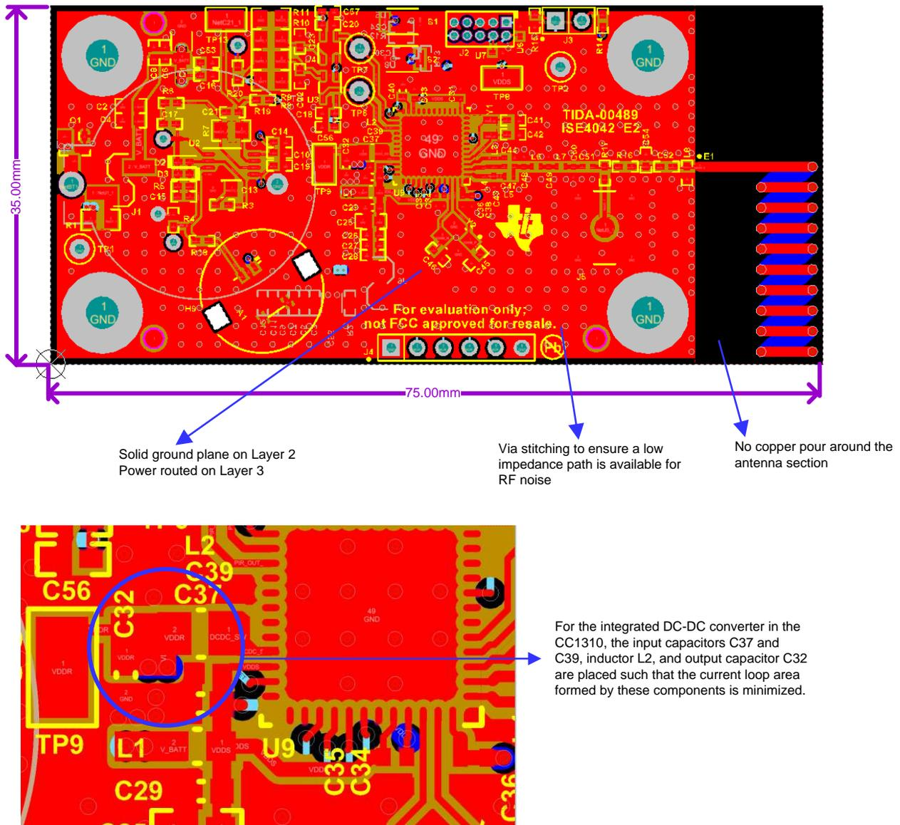
图 35. Low-Power PIR Motion Detector Reference Design Layout Guidelines
