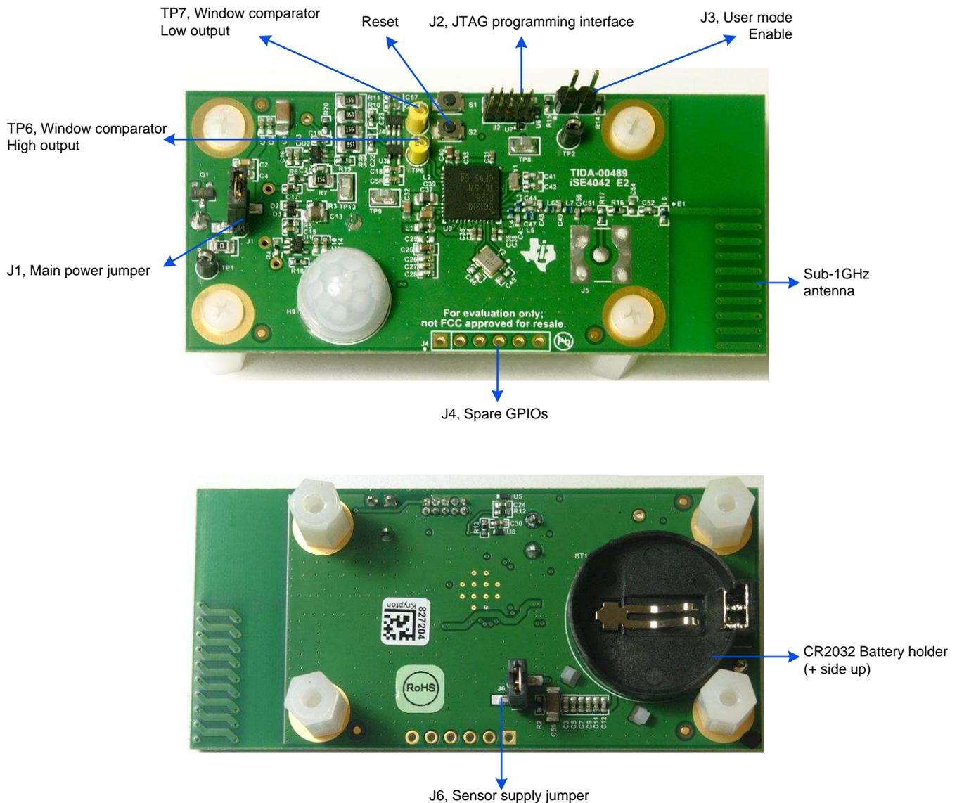
**图 10. Low-Power Wireless PIR Motion Detector Reference Design Hardware Description**
