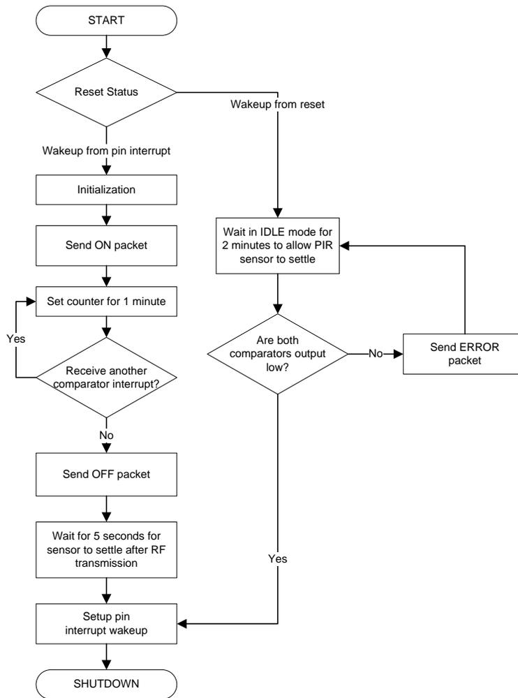
图 9. Wireless PIR Firmware Flowchart
