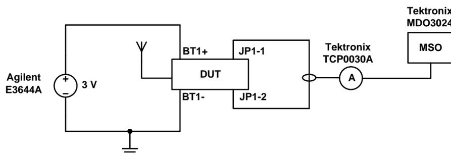
图 18. Test Circuit Used for Measuring Supply Current During Radio Transmission Intervals
