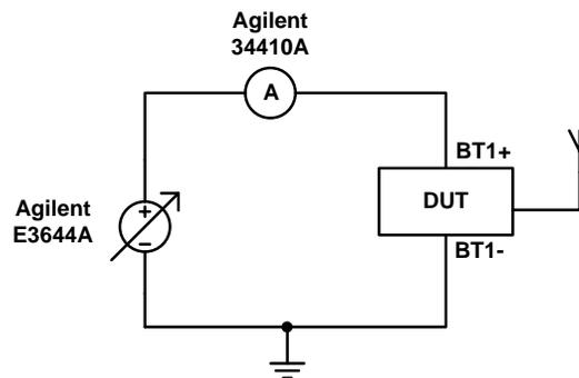
图 17. Test Circuit Used for Measuring Supply Current
