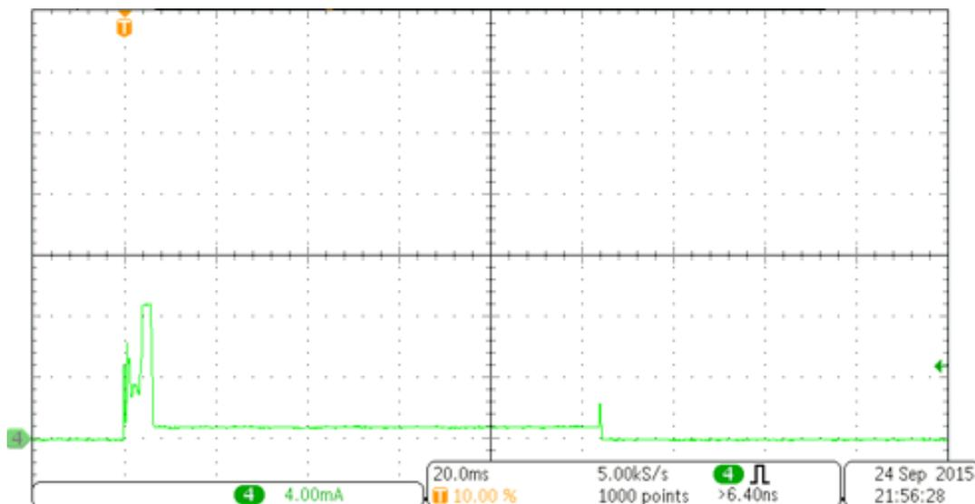
图 23. Radio Transmission Event Supply Current (Full Picture)
