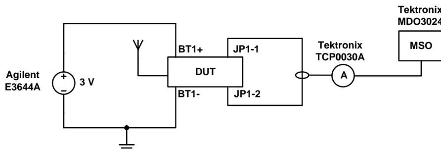
图 18. Test Circuit Used for Measuring Supply Current During Radio Transmission Intervals
