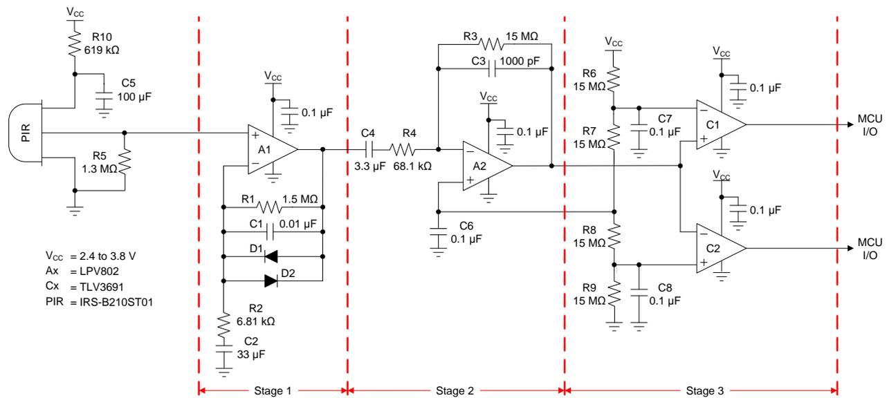
图 5. PIR Motion Sensor Analog Signal Path Schematic
