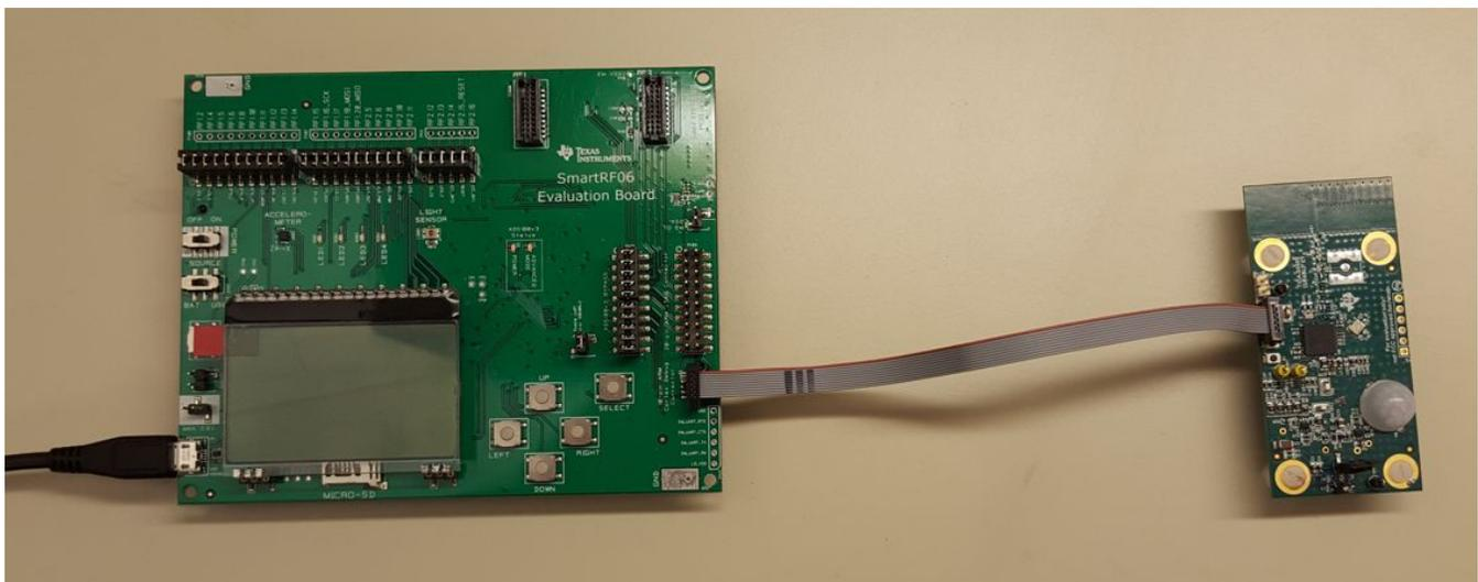
**图 11. Connection of SmartRF06 Evaluation Board and TI Designs Hardware for Programming and Debugging**
