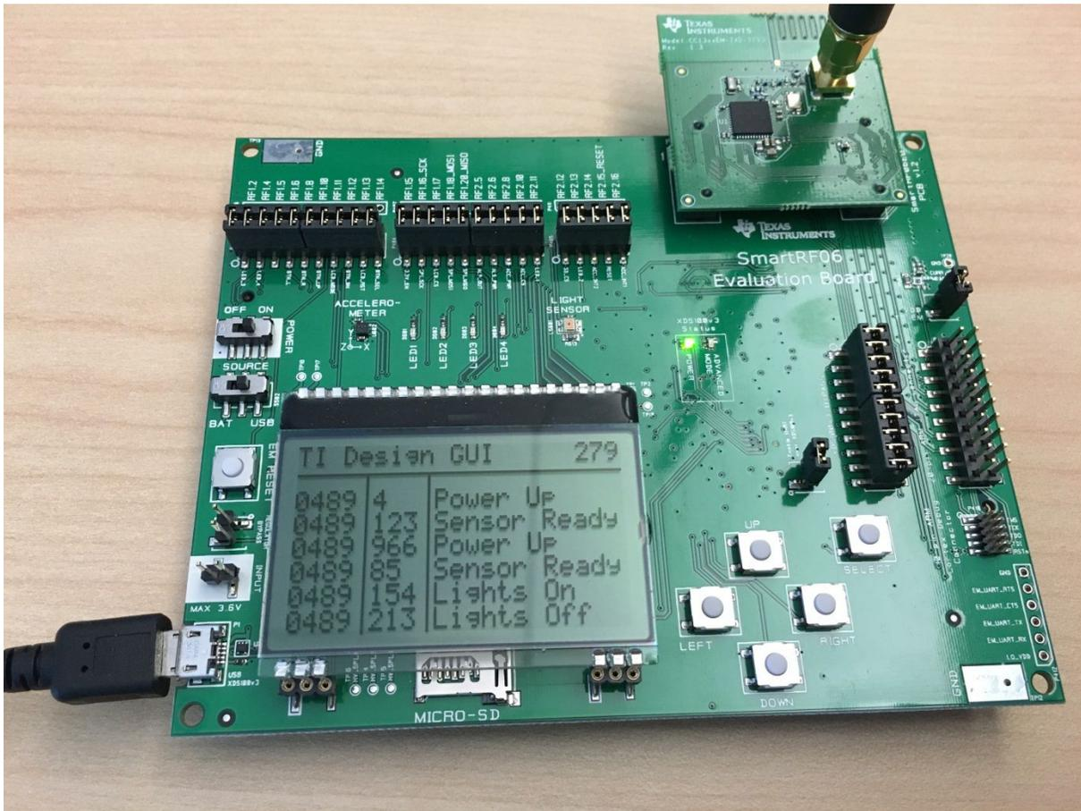
图 12. Building Automation Sub-1GHz Sniffer GUI
