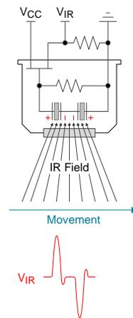
图 4. PIR Motion Sensor Illustration
