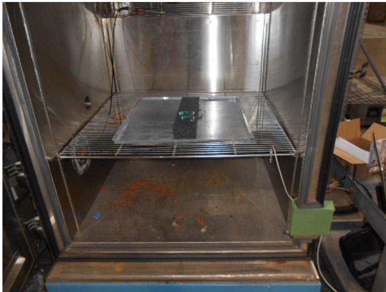
图 19. Wireless PIR Motion Detector Temperature and Humidity Test Setup
