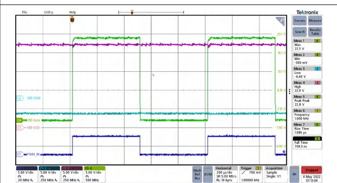
**图 8-9. Gate Waveform Switching 100 nF at 1 kHz.**
