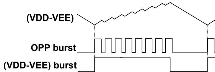
图 7-4. Diagram of Over-Power-Protection with baby burst
