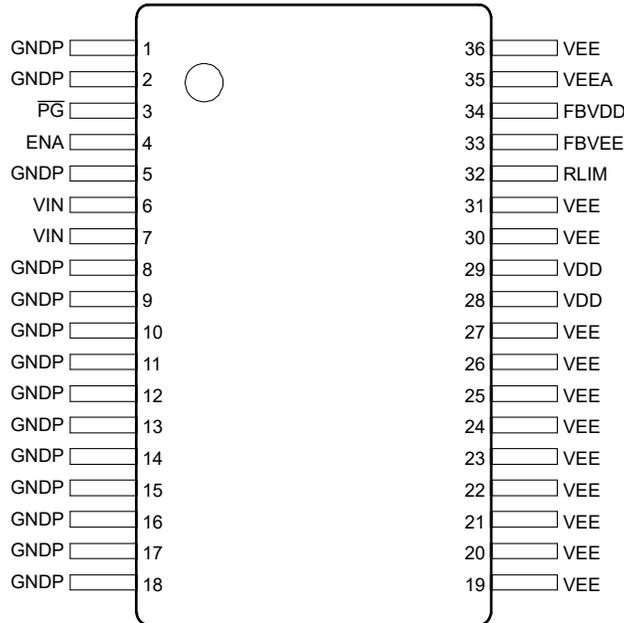
图 5-1. DWN Package, 36-Pin SSOP (Top View)
