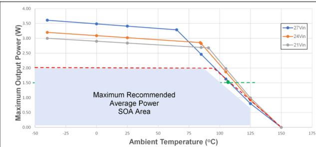
图 6-3. SOA Derating Curves:  $V_{VDD-VEE} = 20\text{ V}$ ,  $V_{COM-VEE} = 5\text{ V}$ , No Load
