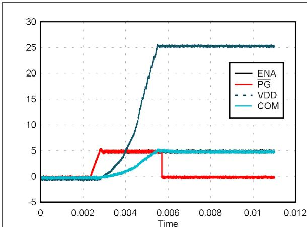
图 6-5. Start-up:  $V_{IN} = 24\text{ V}$ ,  $V_{VDD-VEE} = 25\text{ V}$ ,  $V_{COM-VEE} = 5\text{ V}$ , No Load
