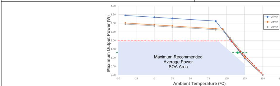
图 6-4. SOA Derating Curves:  $V_{VDD-VEE} = 25\text{ V}$ ,  $V_{COM-VEE} = 5\text{ V}$ , No Load
