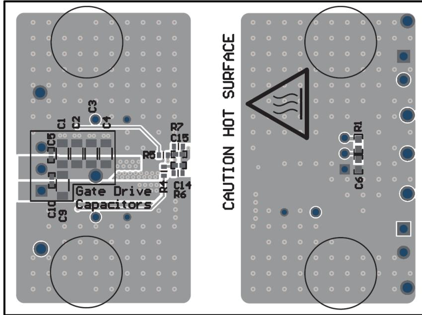
图 8-16. UCC14240-Q1EVM, PCB Bottom Layer, Assembly (Mirrored View)
