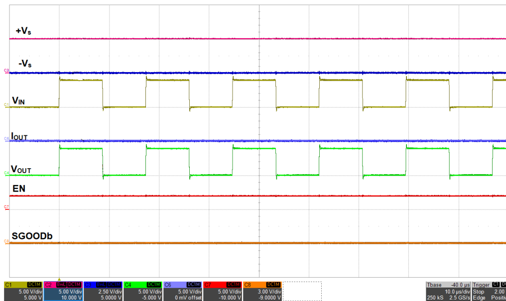
图 9-18. 115.2-Kbps UART Signal Through TPS2661x with V_s of 5 V
