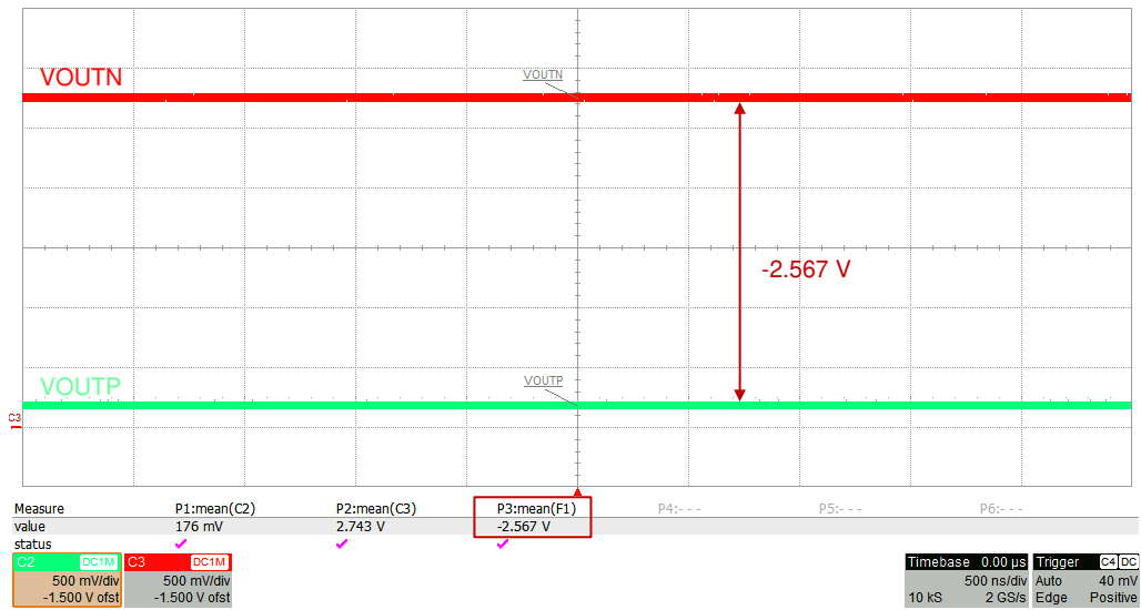
图 6-5. Typical Fail-Safe Output of the AMC3330-Q1
