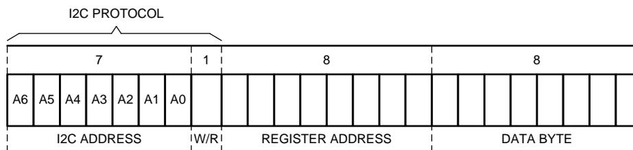
**Figure 9. I<sup>2</sup>C Register Structure**
