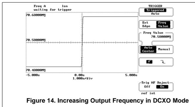
Figure 14. Increasing Output Frequency in DCXO Mode
