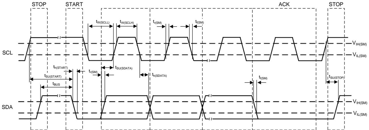
**Figure 8. I<sup>2</sup>C Timing Diagram**
