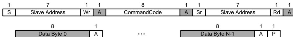
**Figure 12. Block Register Read Programming Sequence**
