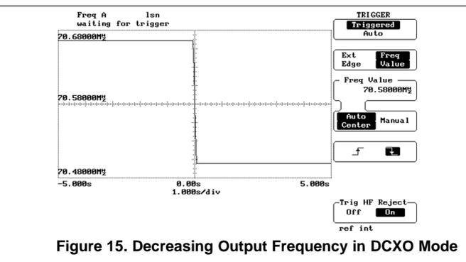
Figure 15. Decreasing Output Frequency in DCXO Mode
