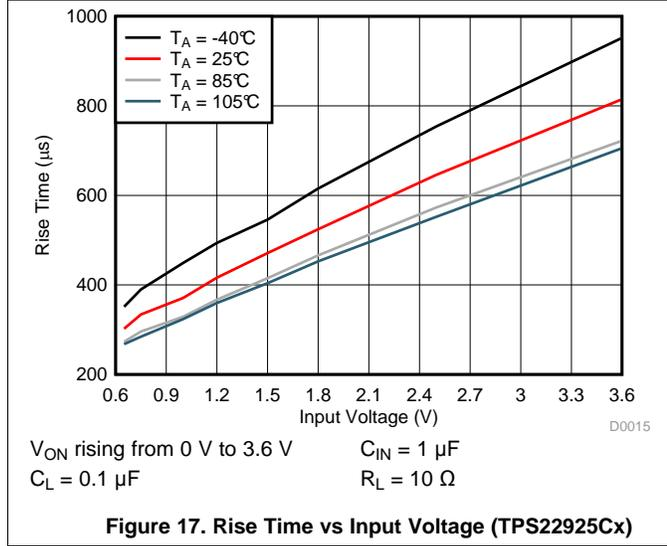
Figure 17. Rise Time vs Input Voltage (TPS22925Cx)
