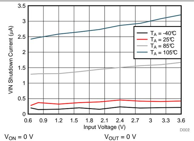
Figure 4. Input Shutdown Current vs Input Voltage
