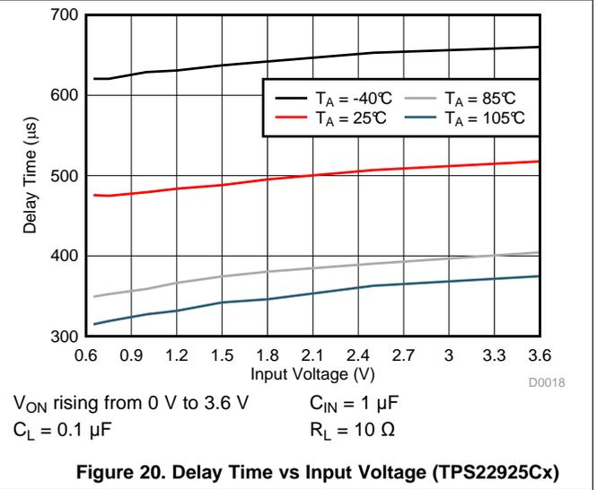
Figure 20. Delay Time vs Input Voltage (TPS22925Cx)
