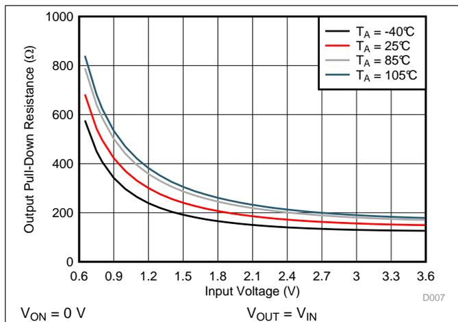
Figure 9. Output Pull-Down Resistance vs Input Voltage
