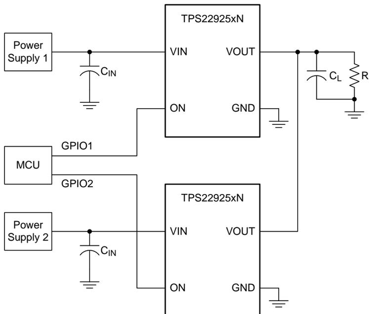
Figure 32. Power Multiplexing with Two TPS22925xN Devices
