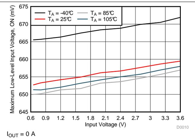
Figure 12. Low-Level Input Voltage vs Input Voltage
