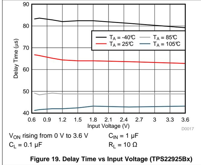
Figure 19. Delay Time vs Input Voltage (TPS22925Bx)
