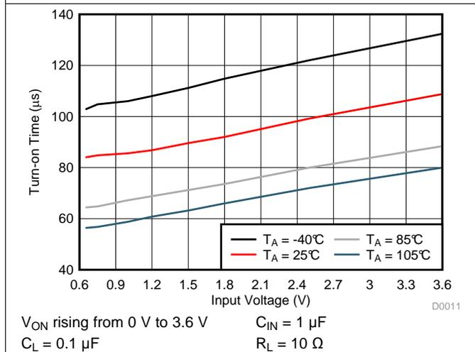
Figure 13. Turn-on Time vs Input Voltage (TPS22925Bx)
