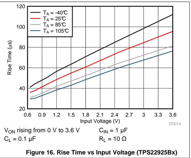
Figure 16. Rise Time vs Input Voltage (TPS22925Bx)
