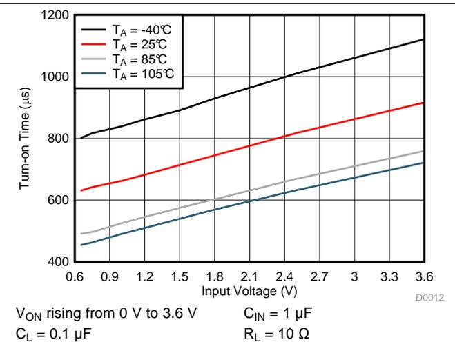
Figure 14. Turn-on Time vs Input Voltage (TPS22925Cx)
