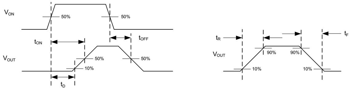
Rise times and fall times of the control signal is 100 ns.
