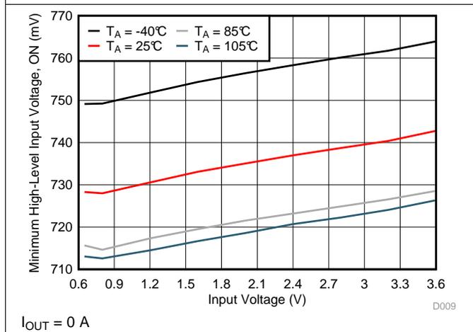
Figure 11. High-Level Input Voltage vs Input Voltage
