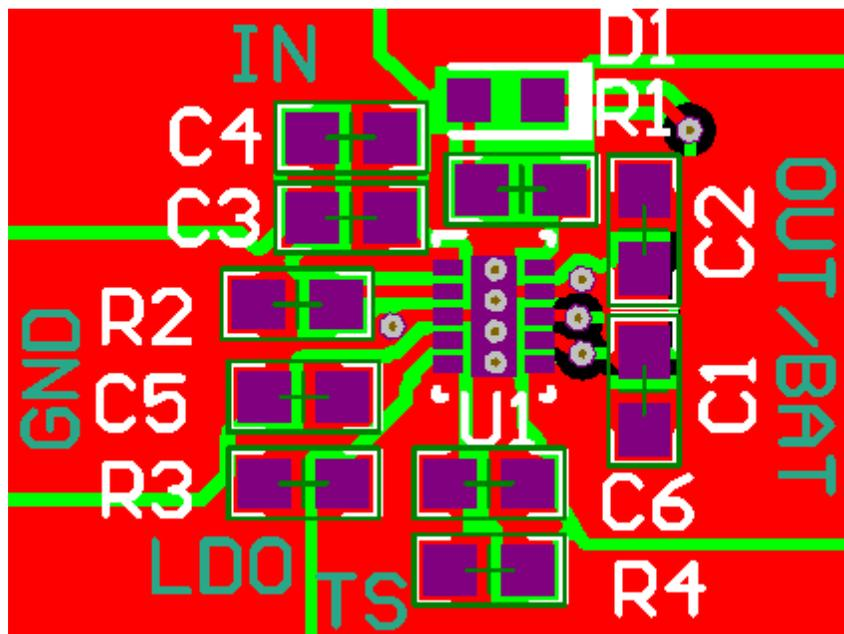
The bottom plane is a ground plane that is connected to the top through vias.
