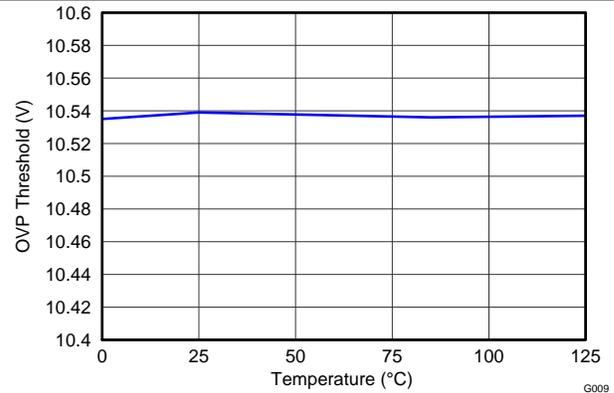
Figure 4. OVP Threshold vs Temperature
