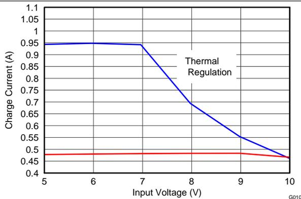
Figure 5. Charge Current vs Input Voltage
