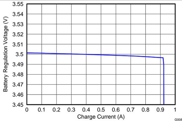
Figure 3. Battery Regulation Voltage vs Charge Current
