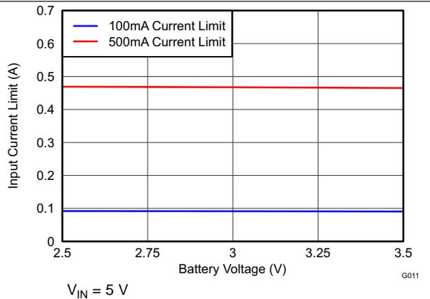
Figure 6. Input Current Limit vs Battery Voltage
