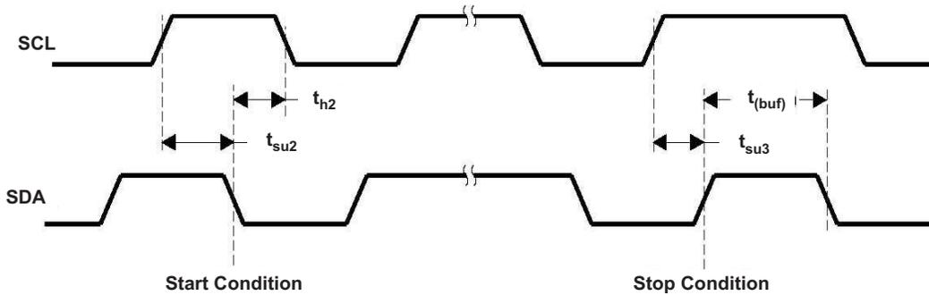
Figure 2. Timing for Start and Stop Conditions
