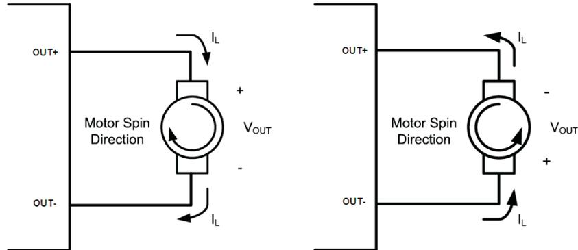
Figure 6. Motor Spin Direction in ERM Motors
