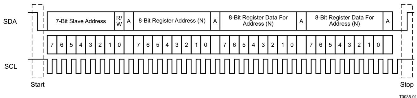
Figure 11. Typical I<sup>2</sup>C Sequence
