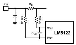
Figure 41. Current Sense Filter
