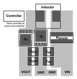
Figure 49. Power Path Layout
