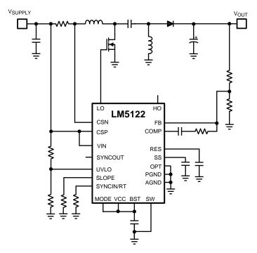
Figure 37. Sepic Converter Simplified Schematic
