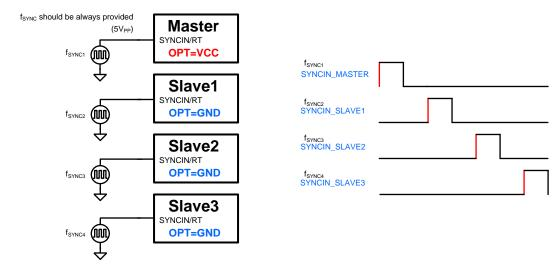
Figure 33. 4-Phase Timing Diagram Individual Clock
