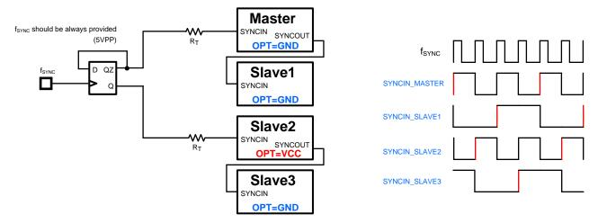
Figure 34. 4-Phase Timing Diagram Daisy Chain
