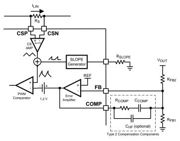
Figure 21. Feedback Configuration and PWM Comparator
