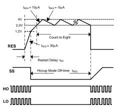
Figure 26. Hiccup Mode Overload Protection
