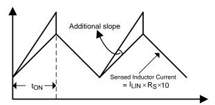
Figure 20. Slope Compensation
