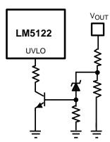
Figure 36. Output Overvoltage Protection
