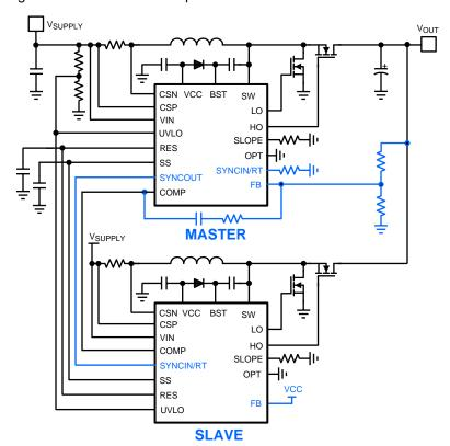
Figure 31. Dual Phase Interleaved Boost Configuration
