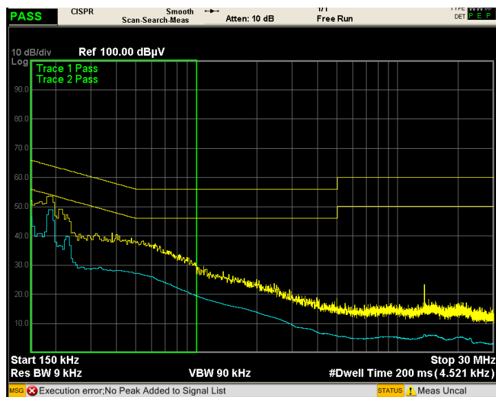
图 2-16. LS LISN - UCC33420 5V/5V Pout = 1.5W
