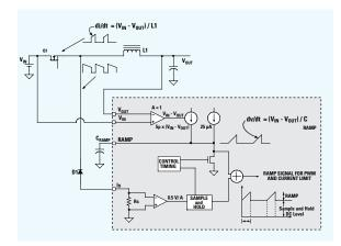
Figure 3. Emulated Current Mode Control Ramp Generator
