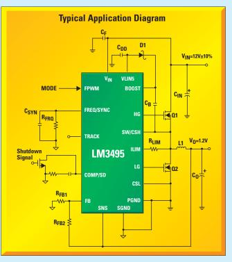
Unique Emulated Peak Current-Mode Control Architecture Enables Jitter-Free Operation with Very Small On-Times
