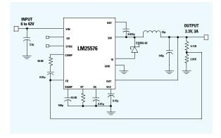
Figure 4. LM25576 Buck Regulator Schematic
