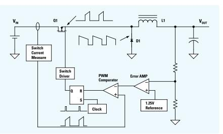
Figure 1. Buck Regulator Using Current Mode Control
