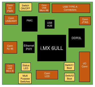
Figure 21. PCB Floor Planning (top)
