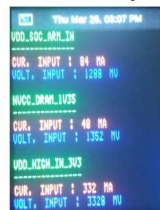
Figure 32. Real-time Current Monitoring with LCD Screen
