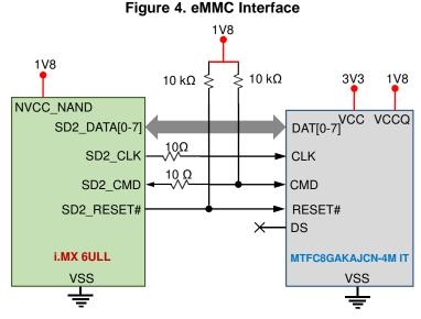
Note: NVCC\_NAND and VCCQ needs to be 1V8 for HS200 Mode. CLK/CMD/DATA lines impedance need to be 50  $\Omega$
