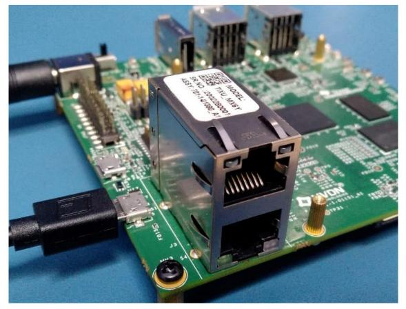
Use TeraTerm or Putty to open a Terminal and get the debug log from the device node if the host PC is running Windows. Change port number according to the COMxx port found in Device Manager for the FTDI chip.
