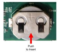
**NOTE:** The voltage of the coin-cell battery (3.0 V nominal) must be above 2.4 V for the supervisor to allow system power-on. If the coin-cell battery voltage is too low, it must be replaced with a fresh battery to continue testing.
