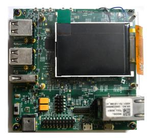
Integrated Power Supply Reference Design for NXP i.MX 6ULL
