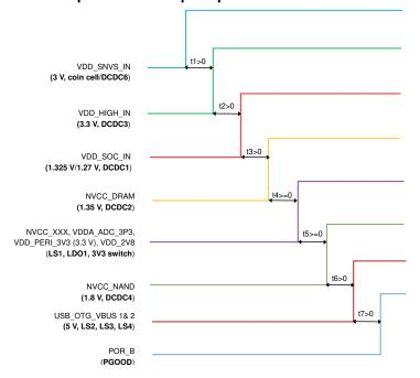
Figure 16. Required Power-Up Sequence for i.MX 6ULL Processor
