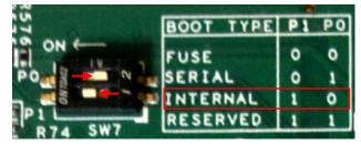
Figure 26. Setting DIP Switch (SW6) for BOOT Config from SD Card
