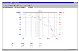
VIN=10V, VOUT2=1V/10A (BW=39.8kHz, PM=60.2D)
