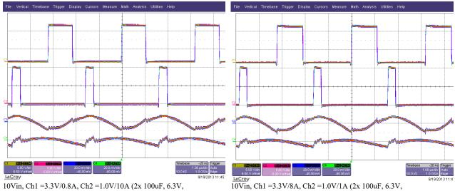
10Vin, Ch1 =3.3V/0.8A, Ch2 =1.0V/10A (2x 100uF, 6.3V, 1210+2x470uF, 4V, 10mohm, 7343), VOUT1=20mVpp
