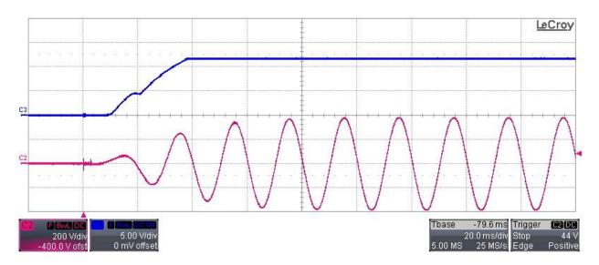
Ch.2: Input voltage (200V/div, 20ms/div, 20MHz BWL) Ch.3: Output voltage (5V/div, 20MHz BWL) Zero load, Vin = 264VAC, 50Hz:
