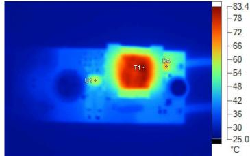
Main Image Markers (230VAC, 50Hz, short circuit on output terminals)
