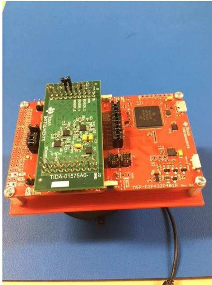
**Figure 9. Mounting Sensor Board**
