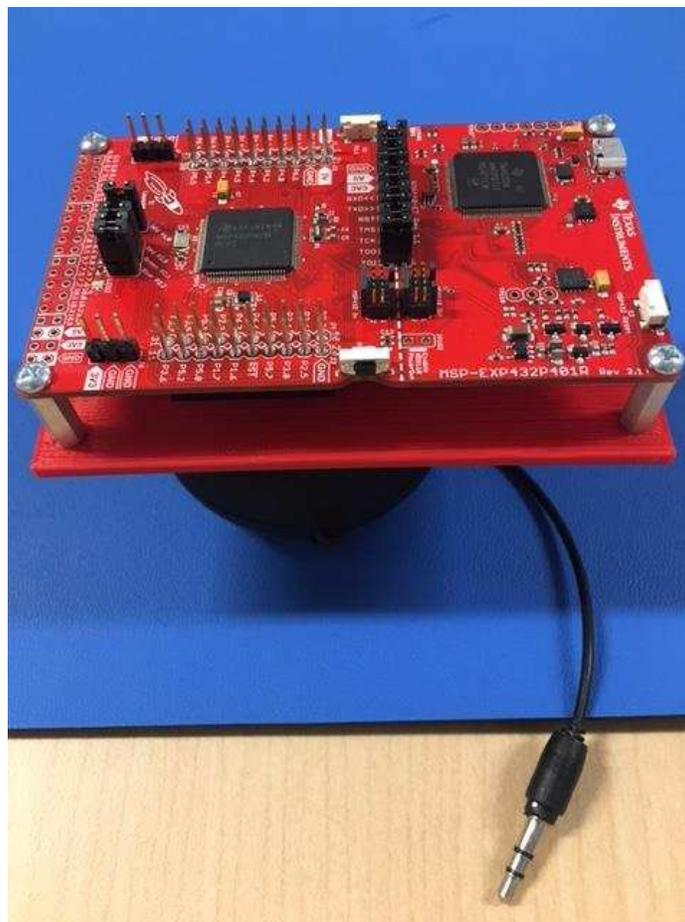
**Figure 8. Mounting LaunchPad™ to Resonator**
