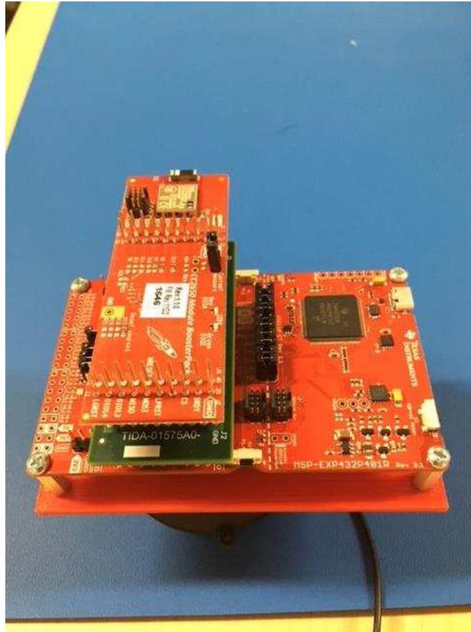
**Figure 10. Mounting BOOSTXL-CC2650MA BoosterPack™**
