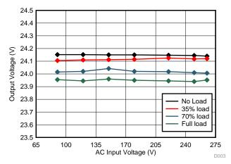
Figure 11. Load Regulation With Load Current
