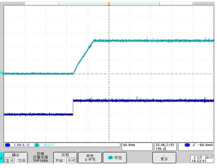
Figure 19. Output Turnon Waveform With CC Load of 1 A
