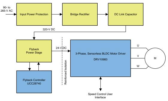
Figure 1. TIDA-01417 System Block Diagram
