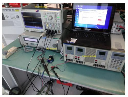
Figure 5. Picture of Test Setup for Flyback Power
