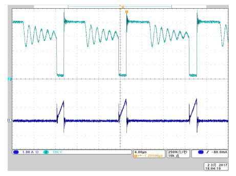
Figure 15. SW Node Waveform and MOSFET Current at V<sub>INAC</sub> = 230-V AC, Full Load
