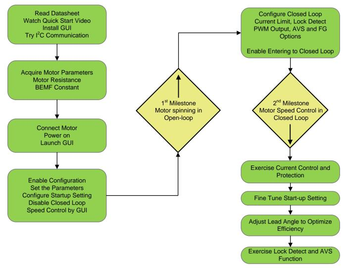
Figure 8. Events for Tuning Motor Parameters for DRV10983
