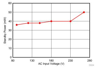
Figure 12. Standby Power With AC Input Variation
