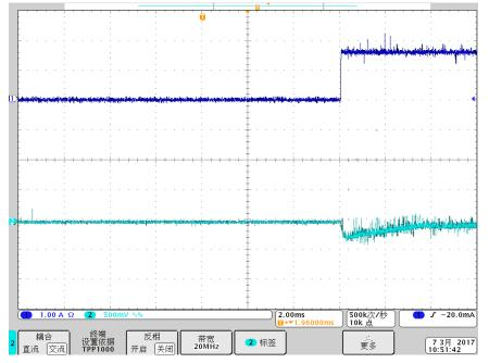
Figure 20. Output Voltage and Current Waveform, Load Transient From 0 to 1.5 A
