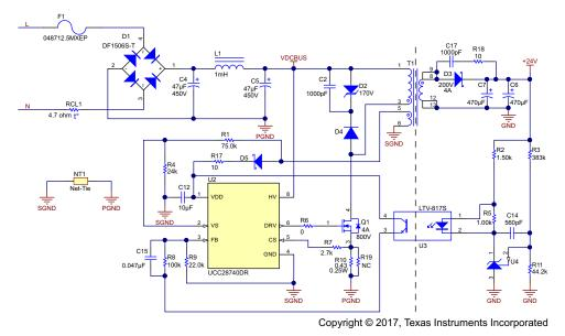
Figure 2. Flyback Power Supply Schematic
