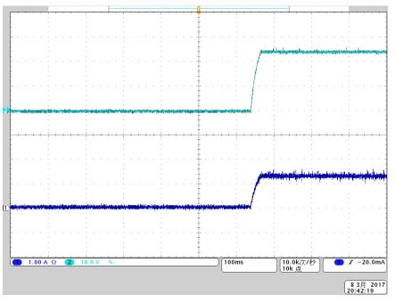
Figure 18. Output Turnon Waveform With Resistive Load of 21.5  $\boldsymbol{\Omega}$
