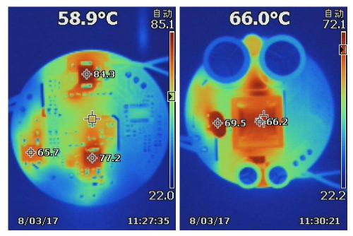
Figure 32. Temperatures at 115-V AC Input and 36-W Output
