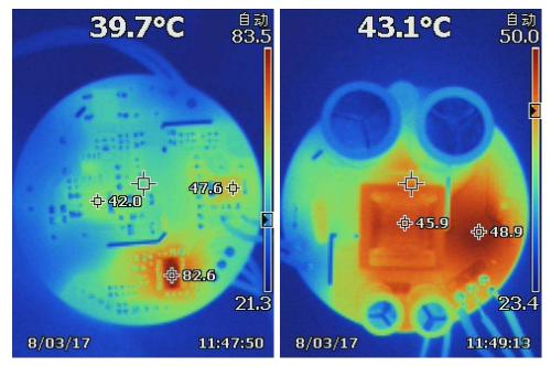
Figure 34. Temperatures for Motor Driver DRV10983
