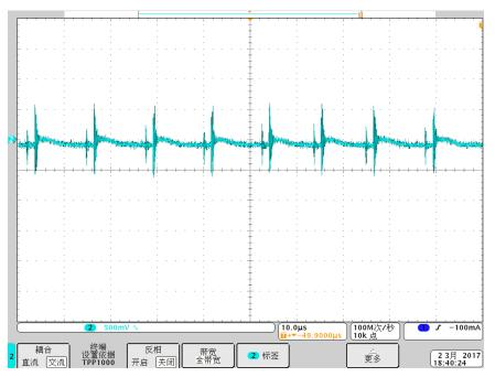
Figure 17. Output Voltage Ripple at  $V_{INAC}$  = 230-V AC, Full Load
