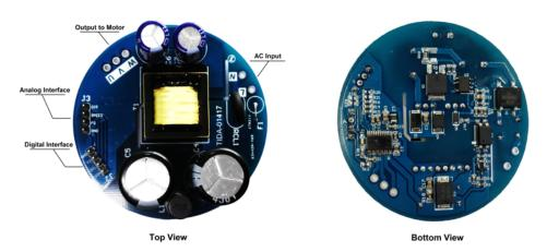
Figure 4. TIDA-01417 PCB Top and Bottom View
