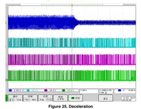
NOTE: Channel 1: Winding current, 2 A/div; Channel 2, 3, 4: U, V, W output voltage, 20 V/div
