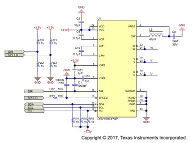
Figure 3. DRV10983 Motor Drive Schematic
