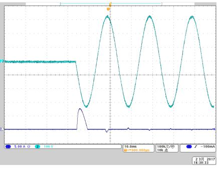
Figure 13. Input Inrush Current at 230-V AC
