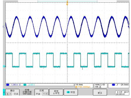
Figure 27 shows the FG signal together with the winding current waveform.
