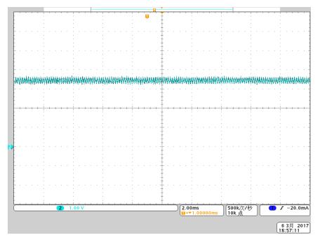
Figure 28. Output Voltage of 3.3 V From Step-Down Regulator of DRV10983
