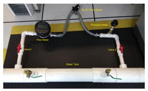
Figure 6. Picture of Test Setup for Motor Driver
