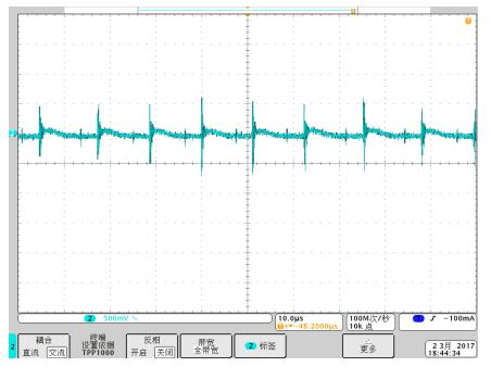
Figure 16. Output Voltage Ripple at V<sub>INAC</sub> = 115-V AC, Full Load
