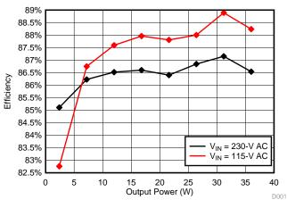
Figure 9. Efficiency versus Output Power
