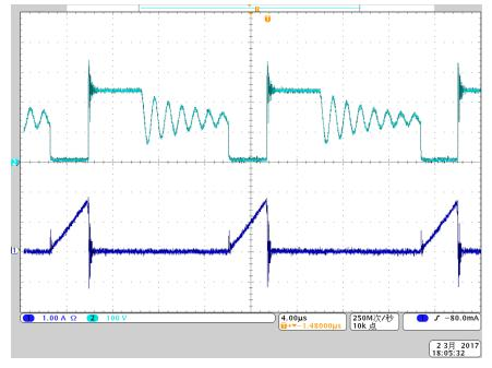
Figure 14. SW Node Waveform and MOSFET Current at V<sub>INAC</sub> = 115-V AC, Full Load
