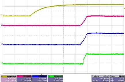
The photo below shows the start up for the board. The outputs are all at full load (VOUT1 @ 200mA, VOUT2 @ 100mA, and VOUT3 @ 200mA). The input voltage is 12V.
