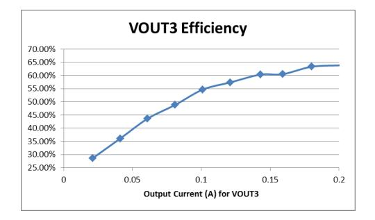
The below plot is an efficiency plot showing the efficiency of the entire system. The three outputs are all loaded simultaneous. The currents are at 20%, 40%, 60%, 80%, and 100% of their full loads.
