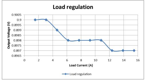
The figures below show output voltage variation of the power rails from no load to full load.
