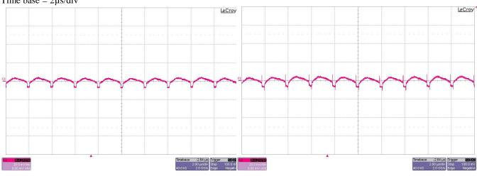
**Rail 2** - Channel 2 – Pink: Output Voltage (20mV/Division; AC Coupled) Time base =  $2\mu$ s/div
