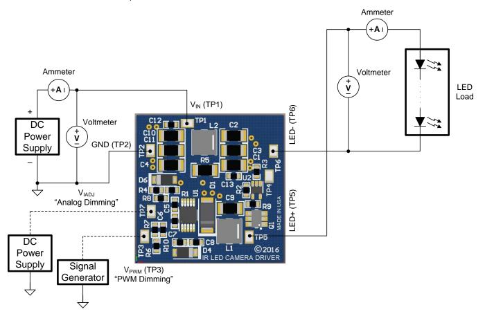
**Figure 6. Test Setup Connections**
