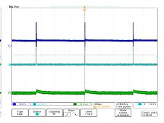
Figure 16. 1% Duty Cycle (IADJ = 0.4 V); Ch1: V<sub>DRN</sub>, Ch2: V<sub>PWM</sub> Ch4: I<sub>LED</sub> (10 mA/div)
