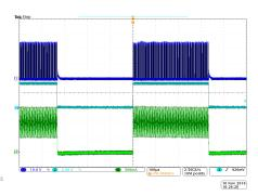
Figure 17. LED Current versus PWM Duty Cycle (0% to 100%)
