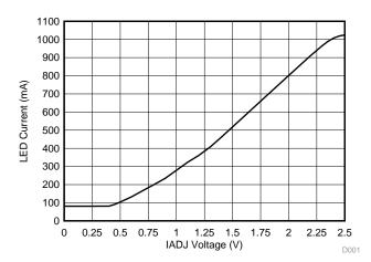
Figure 8. LED Current versus IADJ Voltage (13:1, Minimum Duty Cycle Limited)
