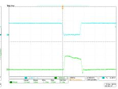
Figure 22. LED Current versus Shunt FET OFF Duty Cycle
