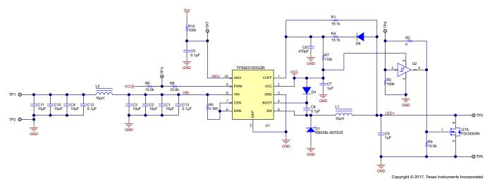
Figure 3. PMP15022 Schematic
