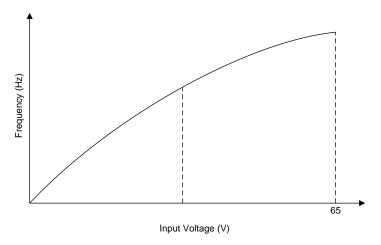
Figure 4. Frequency versus Input Voltage V<sub>IN</sub> (Fixed LED Voltage)
