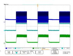
Figure 11. LED Current versus IADJ Voltage (IADJ = 0.4 to 2.5 V)
