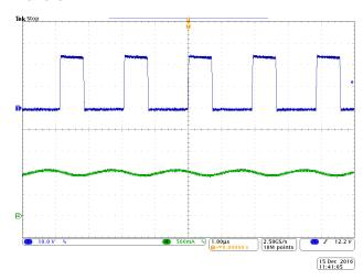
Figure 7. CH 1: Switch Node (DRN) Voltage and CH4: LED Current
