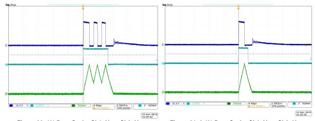
Figure 20. 1% Duty Cycle; Ch1: V<sub>DRN</sub>, Ch2: V<sub>PWM</sub> Ch4: I<sub>LED</sub> (500 mA/div)
