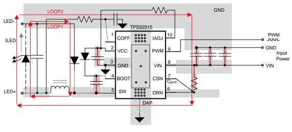
Note: Thermal vias near DAP are required to reduce IC temperature
