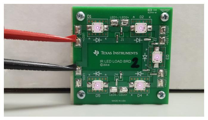
Figure 10. IR LEDs Dimmed to 13:1
