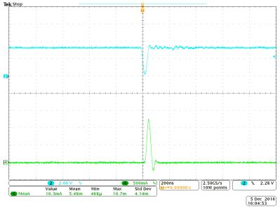
Figure 25. 0.1% Duty Cycle; Ch2: V<sub>TP4</sub> Ch4: I<sub>LED</sub> (500 mA/div)
