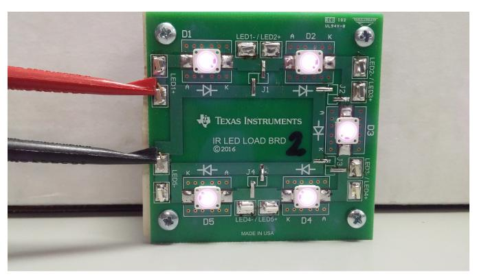
Figure 9. IR LEDs at Full Current
