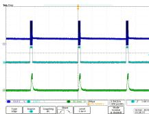
Figure 15. 5% Duty Cycle (IADJ = 0.4 V); Ch1:  $V_{DRN}$ , Ch2:  $V_{PWM}$  Ch4:  $I_{LED}$  (50 mA/div)
