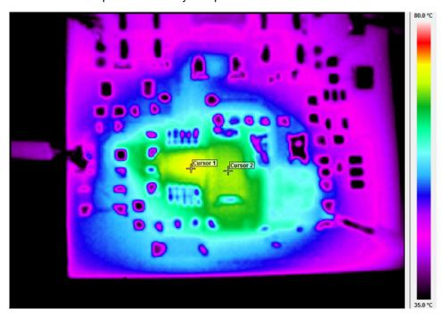
Figure 27. Thermal Scan—Top-View:  $V_{IN} = 24 \text{ V}$ , Five LEDs,  $I_{LED} = 1 \text{ A}$
