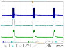
Figure 14. 10% Duty Cycle (IADJ = 0.4 V); Ch1: V<sub>DRN</sub>, Ch2: V<sub>PWM</sub> Ch4: I<sub>LED</sub> (50 mA/div)
