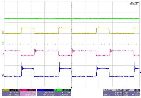
11.2 Voltage stresses on power MOSFETs V<sub>DS</sub> @ 9V<sub>in</sub> and no load
