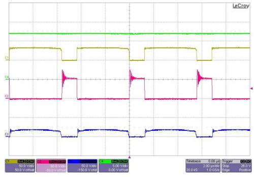
11.4 Voltage stresses on power MOSFETs V<sub>DS</sub> @ 24V<sub>in</sub> and no load
