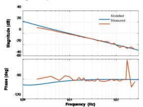
Figure 42. Voltage Loop Modeled Versus Measured Comparison
