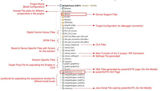
Figure 19. Project Explorer View of Solution Project
