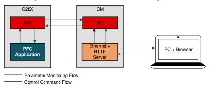
There are two data flows in this test as shown in Figure 50. In the parameter monitoring flow, the three phase current, voltage, and power factors are monitored and shown in HTTP GUI page. In the control command flow, the output voltage reference and command signal (Start PFC --cleartrip) can be set in the GUI page and control the Vienna rectifier.
