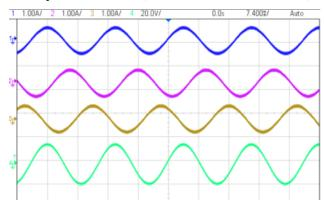
Figure 57. Steady State 208-Vac, IN 600-V DC OUT 1364W, iTHD 0.96%
