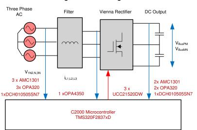
Figure 2. Block Diagram
