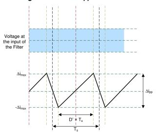
Figure 8. Current Ripple Calculation
