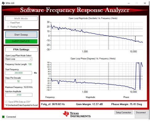
Figure 33. SFRA Run on Closed Current Loop
