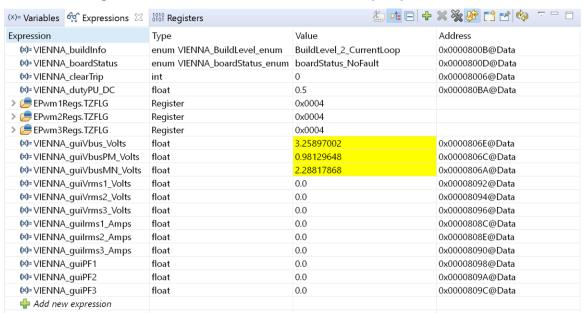
Figure 29. Build Level 2: Closed Current Loop Expressions View
