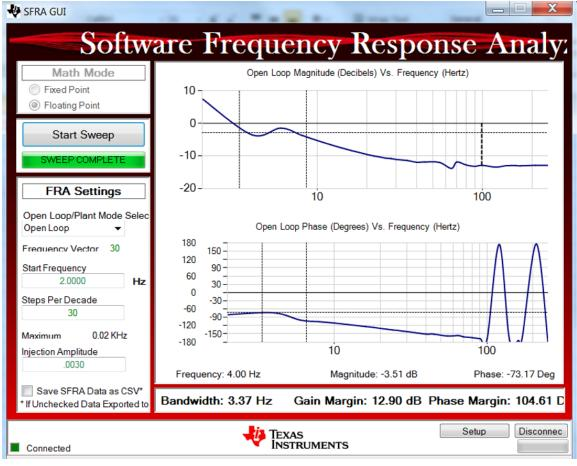
Figure 49. SFRA Run on Balance Voltage Loop
