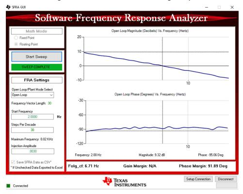
Figure 41. SFRA Run on Closed Voltage Loop
