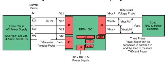
Figure 45. Build Level 4 Hardware Setup Diagram
