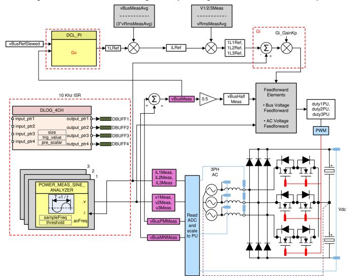
Figure 36. Build Level 3 Control Diagram: Output Voltage Control With Inner Current Loop
