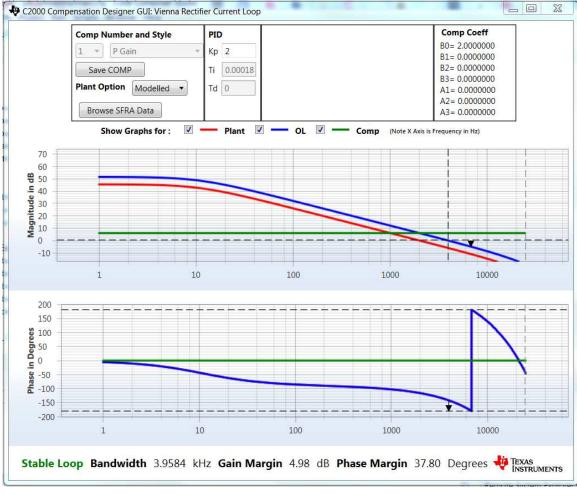
Figure 28. Current Loop Design Using Compensation Designer
