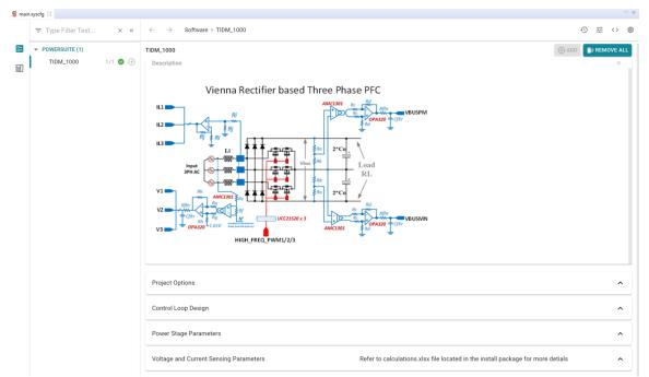
Figure 17. powerSUITE Page for Vienna Rectifier Solution
