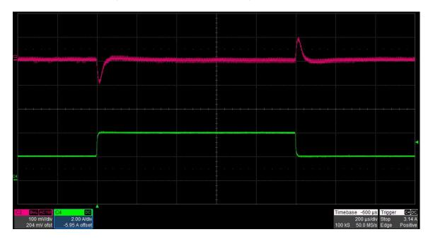
The photo below shows the output voltage (ac coupled) when the load current is stepped between 1A and 4.5A. Vin = 18V. (100mV/DIV, 2A/DIV, 200uS/DIV)
