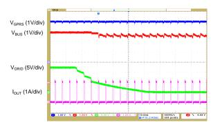
Figure 6. Transition Waveform When Grid Power is Off
