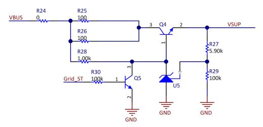
Figure 2. Charger for Super Capacitor
