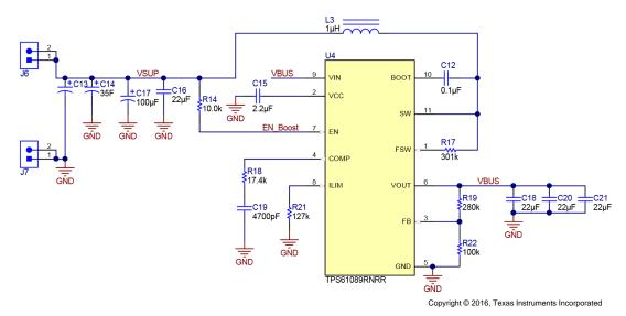
Figure 3. Schematic of Boost Converter Solution
