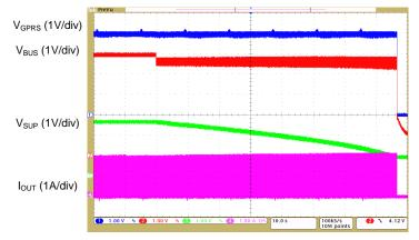
Figure 9. Operating Period of 35F Super Capacitor
