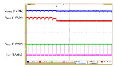
Figure 8. Transition Waveform from Super Capacitor to Battery
