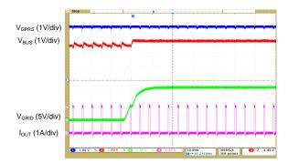
Figure 7. Transition Waveform When Grid Power is On
