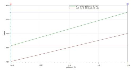
Figure 20. Current Sense DC Sweep Simulation Results
