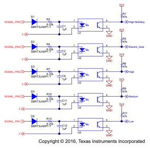
Figure 23. Optocoupler Isolation Schematic
