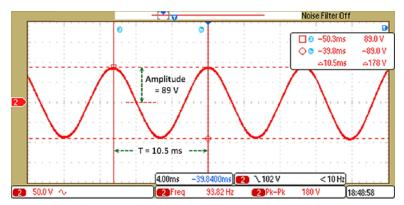
Figure 32. BEMF Oscilloscope Output
