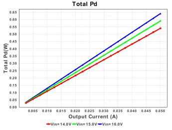
Figure 12. LP2985 Power Dissipation Simulation Results
