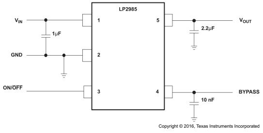
Figure 11. LP2985-33 Application Schematic
