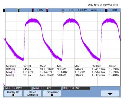
Figure 42. MCU Speed Setting Input From Optocoupler
