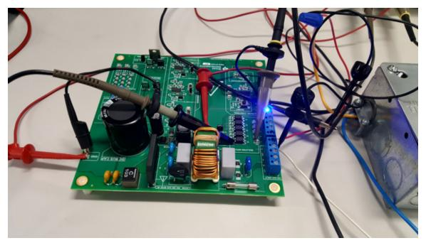
Figure 40. 24-V AC Control Signal Optocoupler Test Setup
