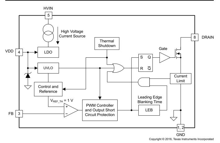
Figure 4. UCC28881 Functional Block Diagram
