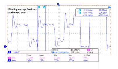
Figure 46. Oscillations in Winding Voltage Feedback for High-Inductance Motor
