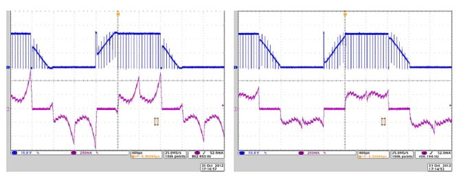
Figure 30. High versus Optimized Flux Threshold Waveforms
