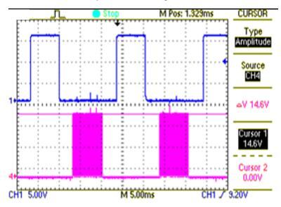
Figure 35. High-Side and Low-Side PWM Input to UCC27714
