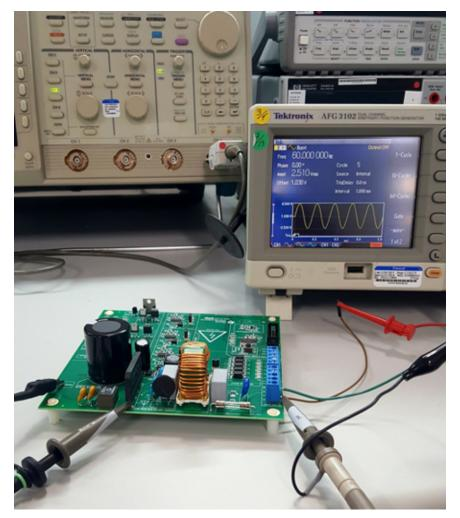
Figure 38. Main Power Supply Testing Setup
