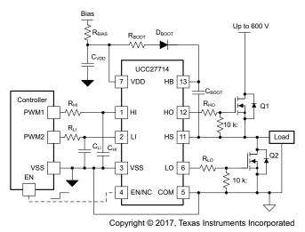
Figure 3. UCC27714 Application Schematic
