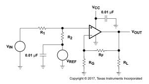
Figure 19. Current Sense Amplifier Setup
