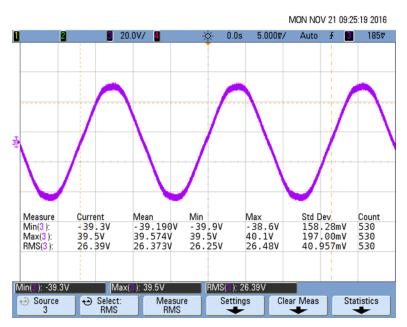
Figure 41. 24-V AC Transformer Optocoupler Input
