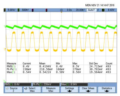
Figure 39. 10 Vp-p Input and DC\_Link Voltage Output
