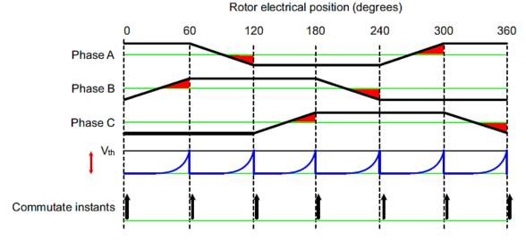
Figure 28. Implementation of Two-Quadrant Uni-Polar PWM
