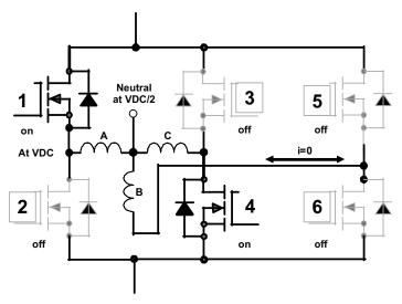
Figure 29. Motor Neutral Voltage During PWM ON
