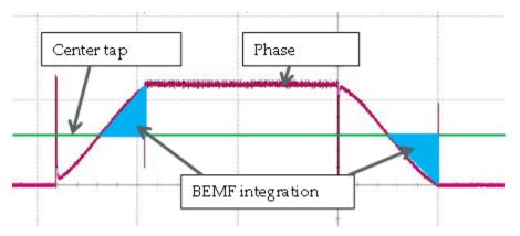
Figure 33. Phase Voltage Waveform Showing BEMF Integration Zones
