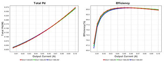
Figure 10. Buck Converter Simulation Output (Power Dissipation and Efficiency)
