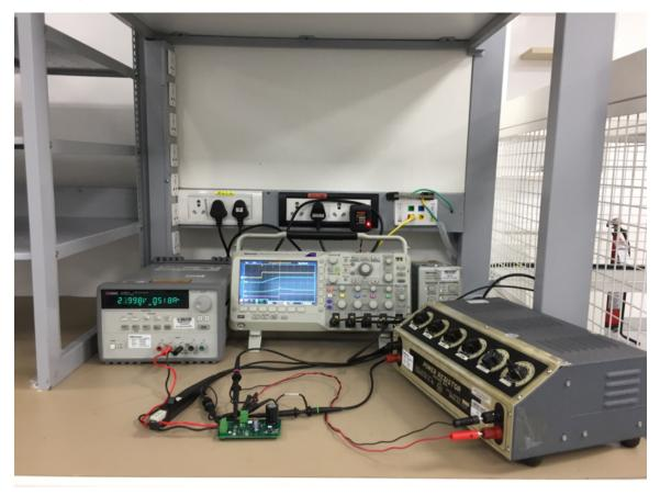
Figure 6. Test Setup
