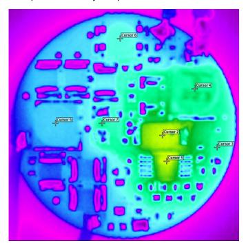
Figure 44. Thermal Scan—Top-View:  $V_{IN} = 14 \text{ V}$ , Two LEDs,  $I_{LED} = 1.25 \text{ V}$
