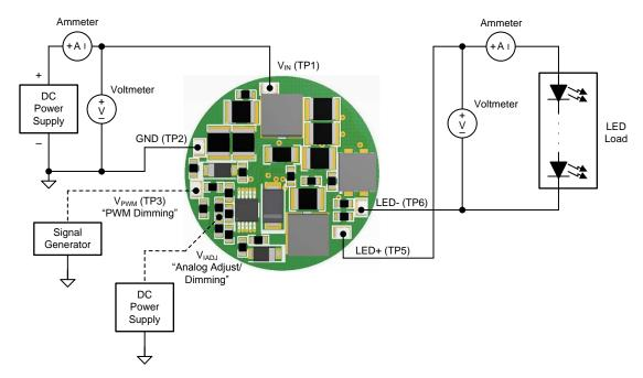
**Figure 6. Test Setup Connections**
