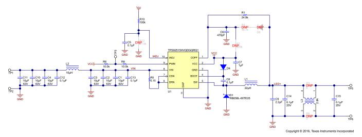
Figure 3. PMP15004 Schematic
