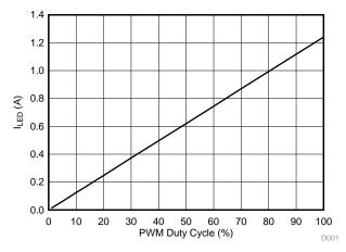
Figure 11. LED Current versus Duty Cycle ( $f_{DIM}$  = 1000 Hz) ( $V_{IN}$  = 14 V, Two LEDs)
