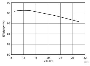
Figure 7. Efficiency versus Input Voltage (Two LEDs)
