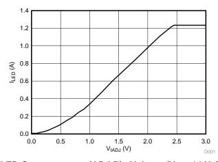
Figure 9. LED Current versus IADJ Pin Voltage ( $V_{IN}$  = 14 V, Two LEDs)
