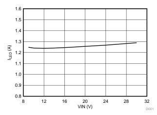
Figure 8. LED Current versus Input Voltage (Two LEDs)
