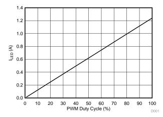
Figure 10. LED Current versus Duty Cycle ( $f_{DIM}$  = 240 Hz) ( $V_{IN}$ = 14 V, Two LEDs)
