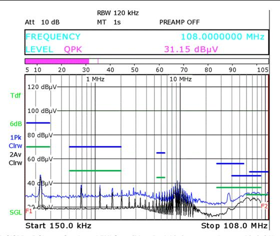
Figure 5. CISPR-25 Class 3 Conducted EMI Scan (Blue: Peak Limits, Green: Average Limits) V<sub>IN</sub> = 14 V, Two LEDs,  $I_{LED} = 1.25 \text{ V}$
