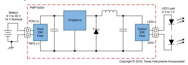
Figure 1. PMP15004 Block Diagram
