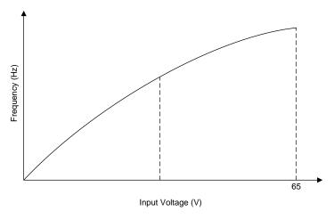
Figure 4. Frequency versus Input Voltage V<sub>IN</sub> (Fixed LED Voltage)
