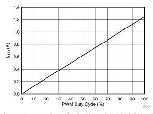
Figure 12. LED Current versus Duty Cycle ( $f_{DIM}$  = 5000 Hz) ( $V_{IN}$  = 14 V, Two LEDs)
