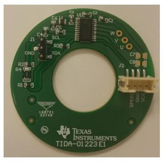
Figure 3. Assembled TIDA-01223 Rev E1 Board
