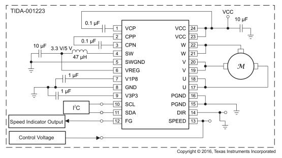
Figure 1. TIDA-01223 Block Diagram
