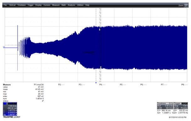
Figure 10. Speed Regulation With Respect to Input Control Voltage (VSP)
