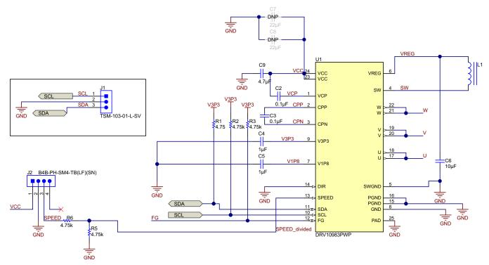
Figure 2. DRV10983 Motor Drive Schematic
