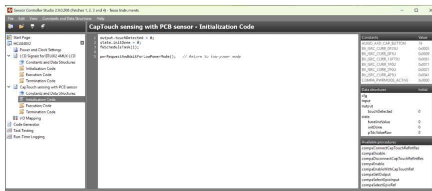
Figure 6-1. SCS Project for CC1312R: CapTouchButton Task (Initialization Code Portion)
