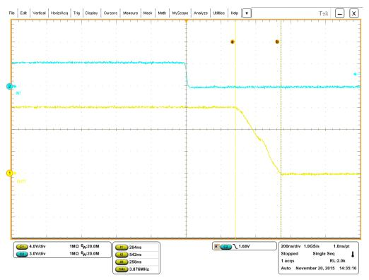
Figure 4: Falling Slew Rate (258 ns)
