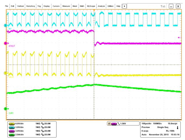
Figure 7: DRV8313 Overcurrent Protection
