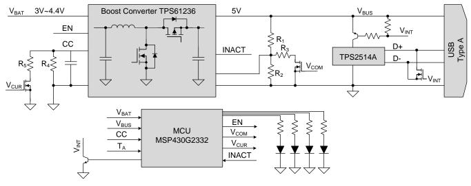
Figure 1: Block Diagram of the Reference-Design
