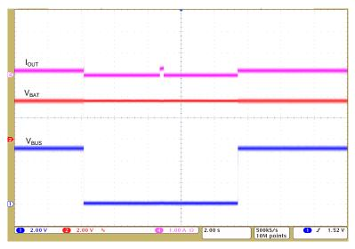
Figure 10: Short Circuit Waveform
