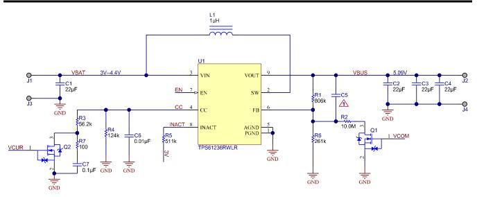
Figure 4: Schematic of the TPS61236
