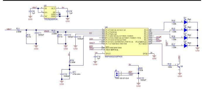
Figure 5: Schematic of the MSP430G2332
