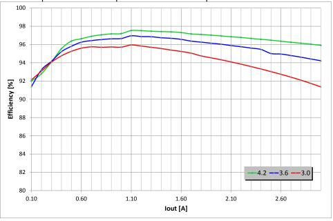
Figure 7: Efficiency of the Reference Design
