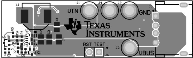
Figure 14 PMP9776 Top Overlay, Top Layer and Top Paste
