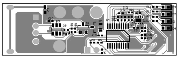
Figure 15 PMP9776 Bottom Overlay and Bottom Layer
