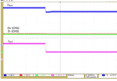
Figure 11: CC Function Operating with IPAD-AIR
