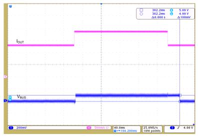
Figure 12: Cable Voltage Drop Compensation
