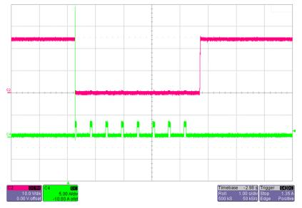
Figure 32. Response During Short Circuit and Auto-Recovery When Short is Removed
