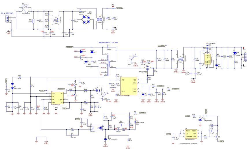
Figure 36. 60-W, High-Efficiency Industrial Power Supply Schematic
