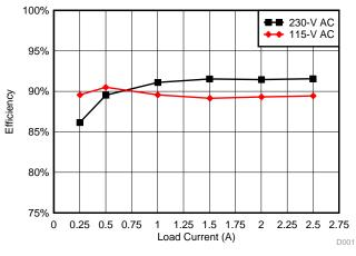
Figure 5. Efficiency versus Output Load Current in CV Mode
