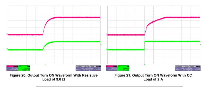
NOTE: Red trace: Output voltage, 10 V/div; Green trace: Output current, 2 A/div.
