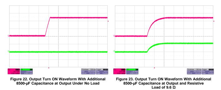
NOTE: Red trace: Output voltage, 10 V/div; Green trace: Output current, 2 A/div.
