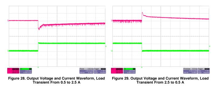
NOTE: Red trace: Output voltage, 100 mV/div, AC coupling; Green trace: Output current, 2 A/div.
