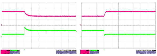
Figure 30. Output Voltage and Current Waveform, Step-Load Transient From 50% Load to 150% Load Figure 31. Output Voltage and Current Waveform, Step-Load Transient from 150% Load to 50% Load
