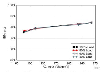
Figure 9. Efficiency Variation With AC Input Voltage Variation in CV Mode
