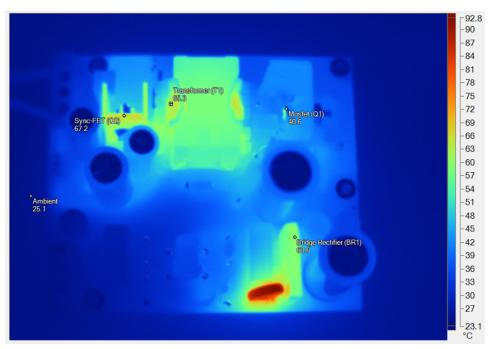
Figure 34. Top-Side Temperatures at 115-V AC Input and 60-W Output
