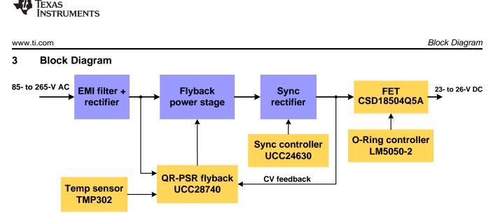
Figure 3. Block Diagram of 60-W DIN Rail Power Supply
