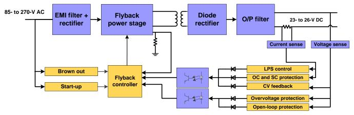
Figure 1. Typical Block Diagram of 60- to 100-W Industrial Power Supply
