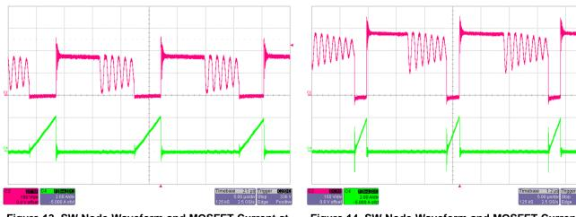
Figure 13. SW Node Waveform and MOSFET Current at V<sub>INAC</sub> = 115-V AC, Full Load
