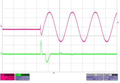
Figure 17. Input Voltage and Input Inrush Current
