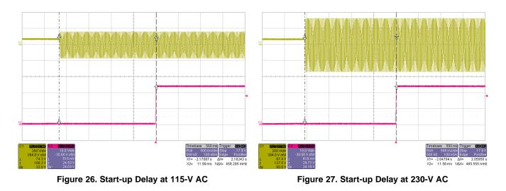
**NOTE:** Red trace: Output voltage, 10 V/div; Yellow trace: Input AC voltage: 200 V/div.
