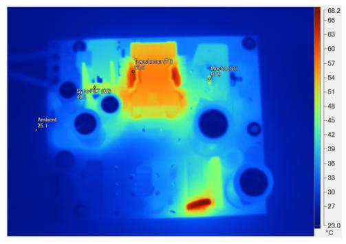
Figure 35. Top-Side Temperatures at 230-V AC Input and 91.2-W Output
