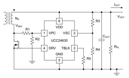
Figure 4. UCC24630 Circuit Component Design
