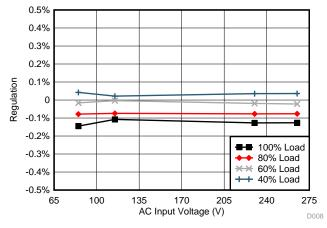
Figure 10. Output Voltage Variation With AC Input Voltage Variation in CV Mode
