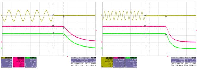
Figure 24. Hold-Up Time at 115-V AC
