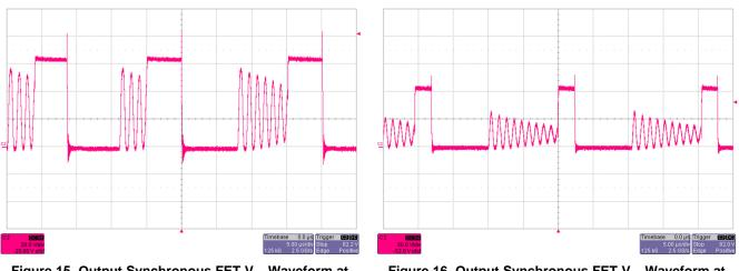
Figure 15. Output Synchronous FET V\_{DS} Waveform at V\_{INAC} = 115-V AC, Full Load
