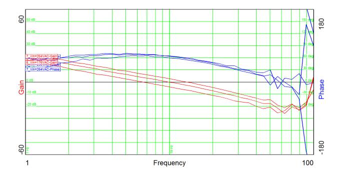
$\begin{array}{lll} \text{Input Voltage} & = 176 \text{VAC} \\ \text{LED Current} & = 0.71 \text{A} \\ \text{LED Voltage} & = 233 \text{V} \\ \text{Phase margin} & = 69^{\circ} \\ \text{Bandwidth} & = 7 \text{Hz} \\ \end{array}$
