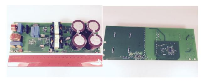
Load: 2 LED strings in parallel. Max. LED current each string: 0.35A
