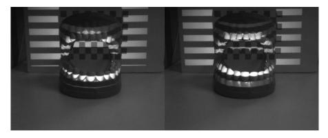
Figure 41 Non-inverted and inverted horizontal Gray code pattern 4 capture
