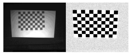
Figure 5 Printed calibration board and projected calibration board position 4
