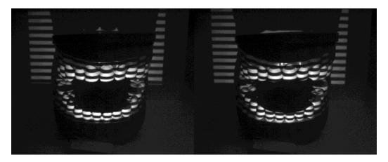
Figure 28 Non-inverted and inverted horizontal Gray code pattern 6 capture
