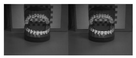
Figure 43 Non-inverted and inverted horizontal Gray code pattern 6 capture
