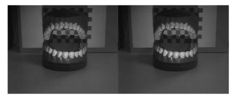
Figure 43 Non-inverted and inverted horizontal Gray code pattern 7 capture
