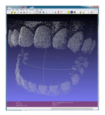
Figure 36 Isometric view of point-cloud from 3D scan
