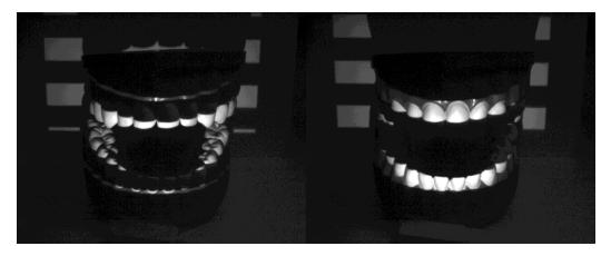
Figure 26 Non-inverted and inverted horizontal Gray code pattern 4 capture
