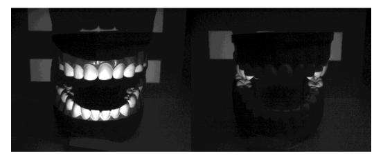
Figure 25 Non-inverted and inverted horizontal Gray code pattern 3 capture
