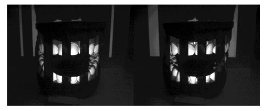
Figure 18 Non-inverted and inverted vertical Gray code pattern 5 capture
