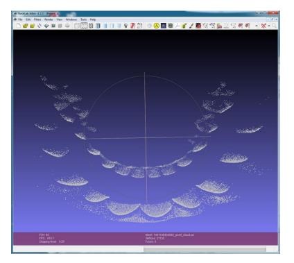
Figure 35 Top view of point-cloud from 3D scan
