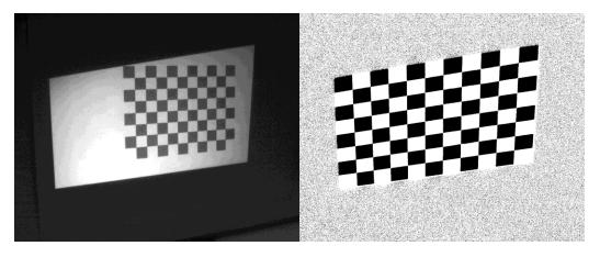
Figure 6 Printed calibration board and projected calibration board position 5
