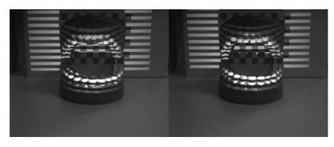
Figure 42 Non-inverted and inverted horizontal Gray code pattern 5 capture
