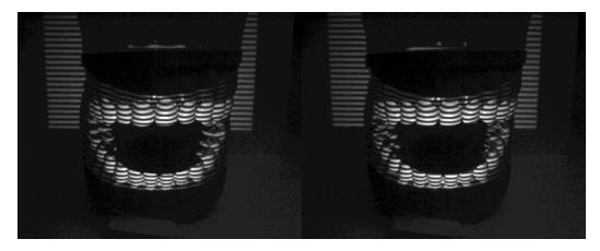
Figure 29 Non-inverted and inverted horizontal Gray code pattern 7 capture
