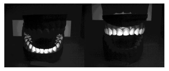
Figure 23 Non-inverted and inverted horizontal Gray code pattern 1 capture
