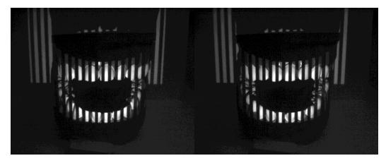
Figure 20 Non-inverted and inverted vertical Gray code pattern 7 capture
