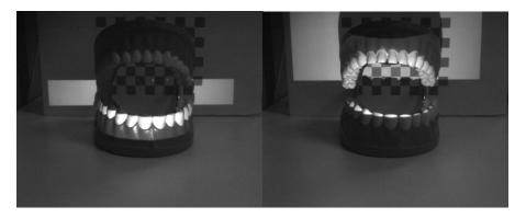
Figure 38 Non-inverted and inverted horizontal Gray code pattern 1 capture
