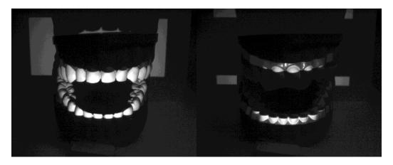
Figure 24 Non-inverted and inverted horizontal Gray code pattern 2 capture
