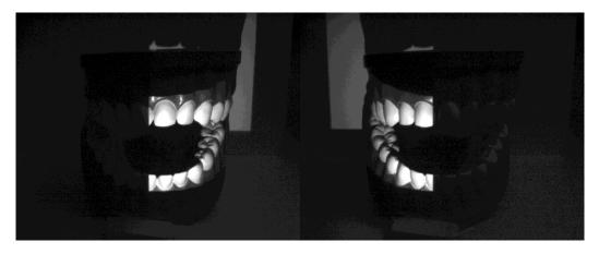
Figure 14 Non-inverted and inverted vertical Gray code pattern 1 capture
