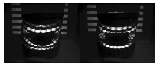
Figure 27 Non-inverted and inverted horizontal Gray code pattern 5 capture
