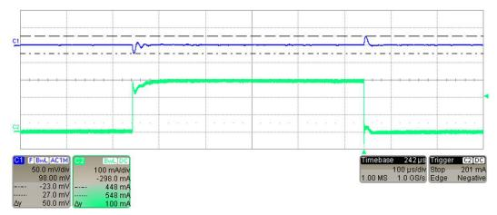
Figure 48. V\_CORE, VOUT = 1.06 V, IOUT\_STEP = 300 mA
