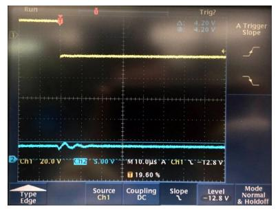
Figure 65. Max Overshoot = 4.2 V Protects Circuits Downstream
