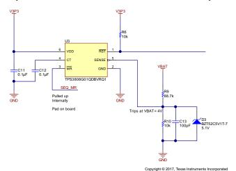
Figure 9. TPS3808-Q1 Voltage Supervisor
