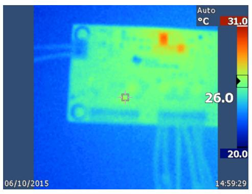
Figure 58. TPS54116-Q1 IC, No Load, Steady State
