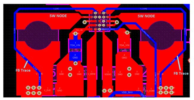
Figure 72. Routing Feedback Traces Around Switch Nodes
