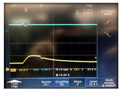
Figure 68. TVS Circuit Clamps Voltage to 31.6 V
