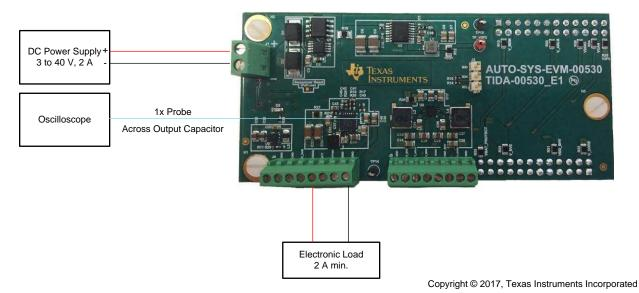
Figure 20. DC-DC Converter Output Voltage Ripple and Thermal Measurement Setup
