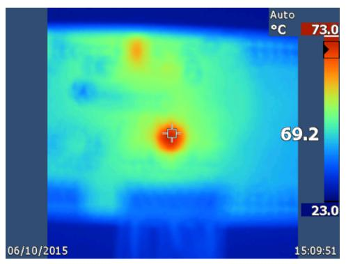
Figure 57. LP8731 IC, All Four Rails Full Load, Steady State
