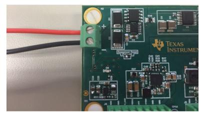
Figure 13. Board Input Terminal
