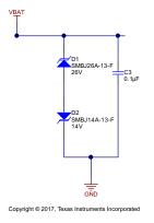
Figure 6. Input Transient Protection
