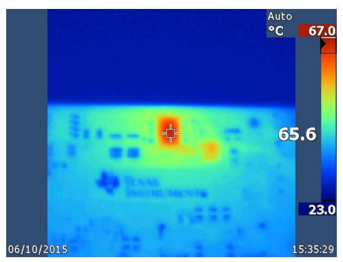
Figure 54. LM53603 (Wide-VIN Buck) IC, Full Load, Steady State
