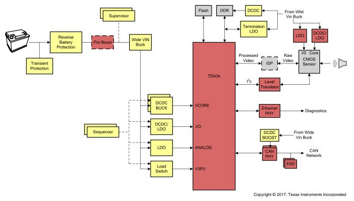
Figure 1. Example TDA3x-Based Mono Front Camera Block Diagram
