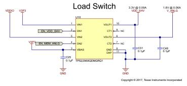
Figure 10. Load Switch Schematic
