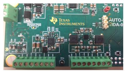
Figure 15. Screw Terminals for Supply Outputs
