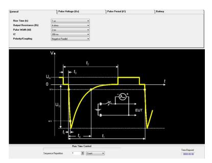
Figure 26. AutoStar Setup for Pulse 1
