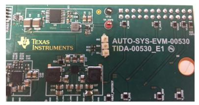
Figure 14. I<sup>2</sup>C Header
