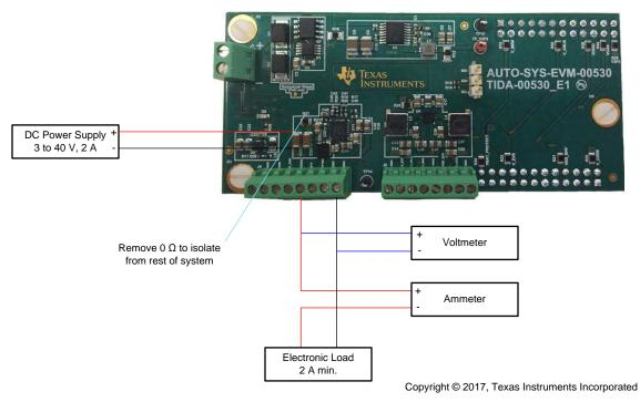
Figure 23. Load Regulation Measurement Setup
