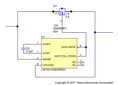
Figure 5. Reverse Battery Input Protection
