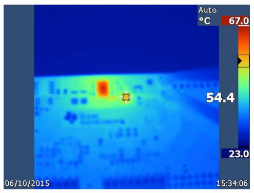
Figure 55. LM53603 (Wide-VIN Buck) Inductor, Full Load, Steady State
