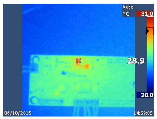
Figure 53. LM53603 (Wide-VIN Buck) IC, No Load, Steady State
