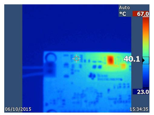
Figure 52. LM74610 (Reverse Polarity Protection) FET, Full Board Load, Steady State
