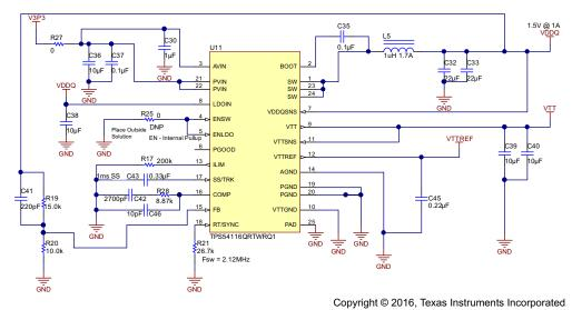
Figure 12. TPS54116-Q1 VDDQ DDR Regulator
