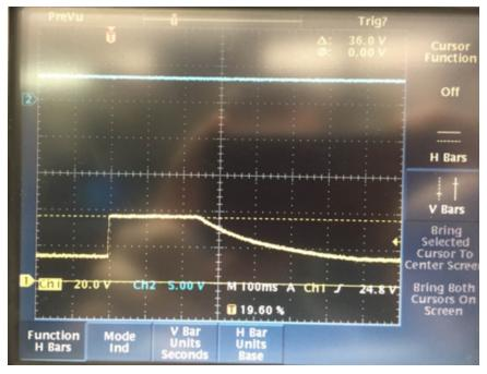
Figure 71. Wide V<sub>IN</sub> Output Undisturbed During Load Dump Pulse
