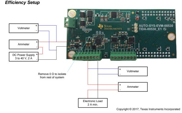
Figure 22. DC-DC Efficiency Measurement Setup
