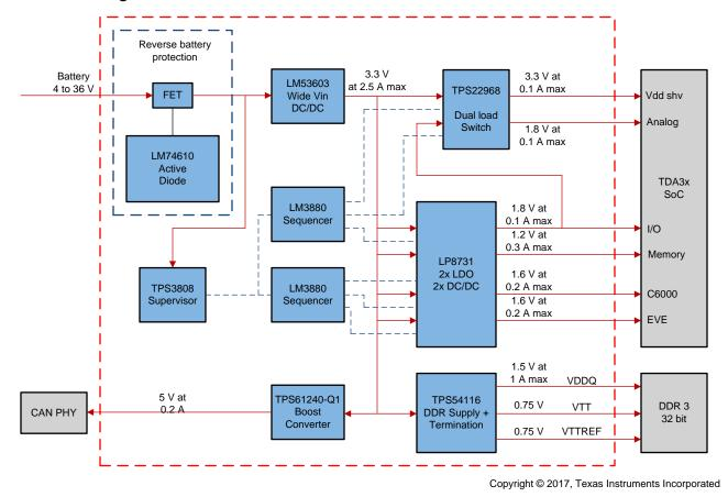
Figure 2. Power Solution for TDA3x Based Systems
