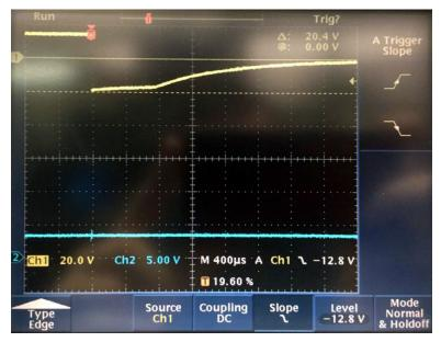
Figure 64. TVS Circuit Clamps the Negative Voltage to -20.4 V
