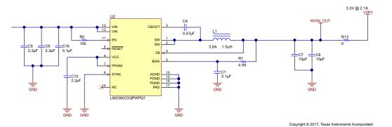
Figure 7. LM53603-Q1 Wide Input Voltage Buck
