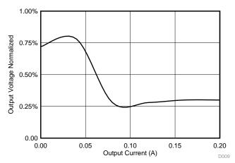
Figure 35. VCAN Load Regulation 0 to 0.2 A ( $V_{IN} = 3.3 V$ )
