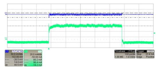
Figure 50. V\_CAN, VOUT = 5 V, IOUT\_STEP = 50 mA
