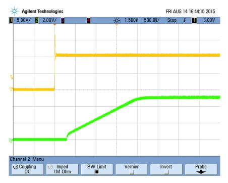
Figure 9 Power up into no load at 10V input
