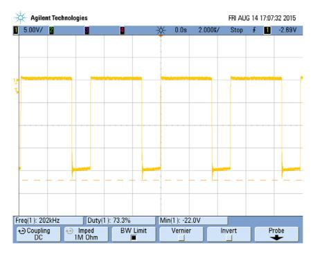
Figure 13 Output diode anode (+) to cathode (-) voltage at 15V input, full load
