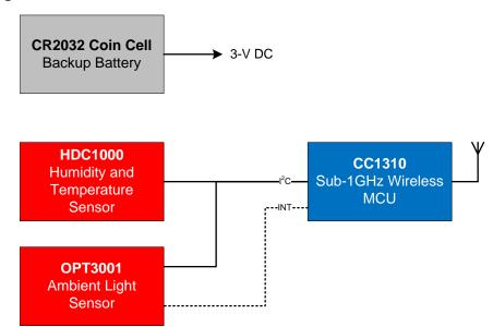
Figure 2. Interrupt-Based Ambient Light and Environment Sensor Node for Sub-1GHz Networks Reference Design System Block Diagram
