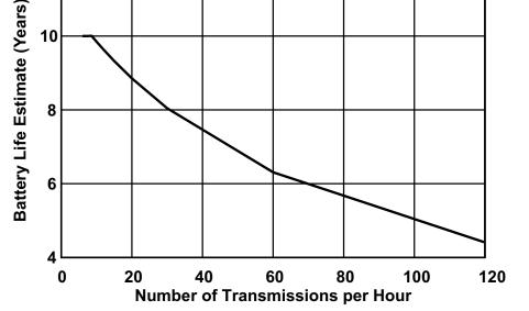
Figure 17. Battery Life Estimation versus Number of Transmissions per Hour for TIDA-00758
