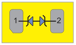
Figure 7. TPD1E10B06 Functional Block Diagram
