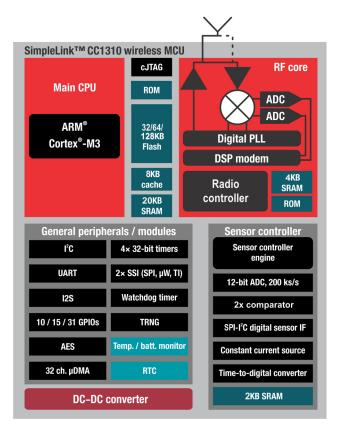
Figure 3. CC1310 Functional Block Diagram
