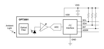
Figure 5. OPT3001 Functional Block Diagram
