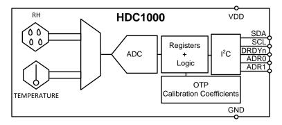
Figure 6. HDC1000 Functional Block Diagram
