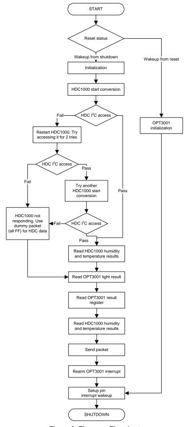
**Figure 8. Firmware Flowchart**
