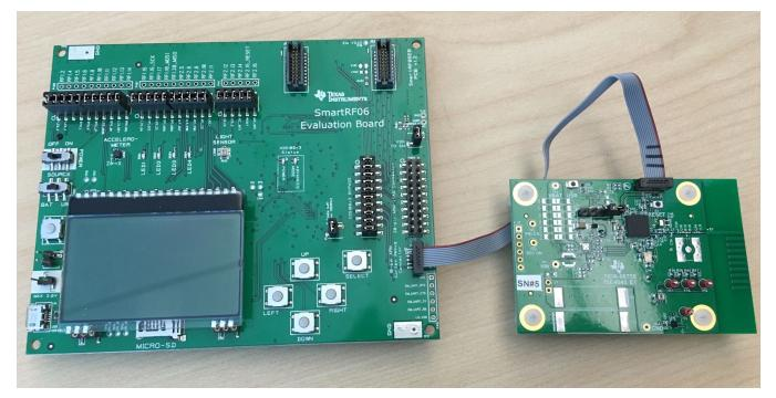
Figure 10. Connection of SmartRF06 EVM and TI Designs Hardware for Programming and Debugging
