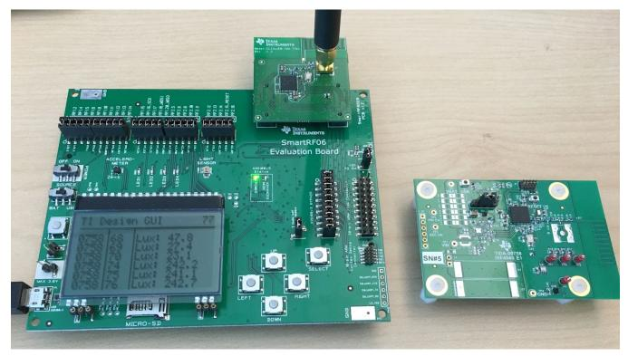
Figure 11. Sniffer Application Firmware Running on the SmartRF06 EVM With TIDA-00758 and TIDA-00488 Reference Designs
