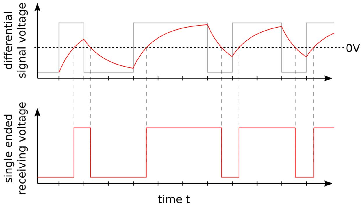
**Figure 3. Top: Theoretical (gray) and real (red) differential signal
