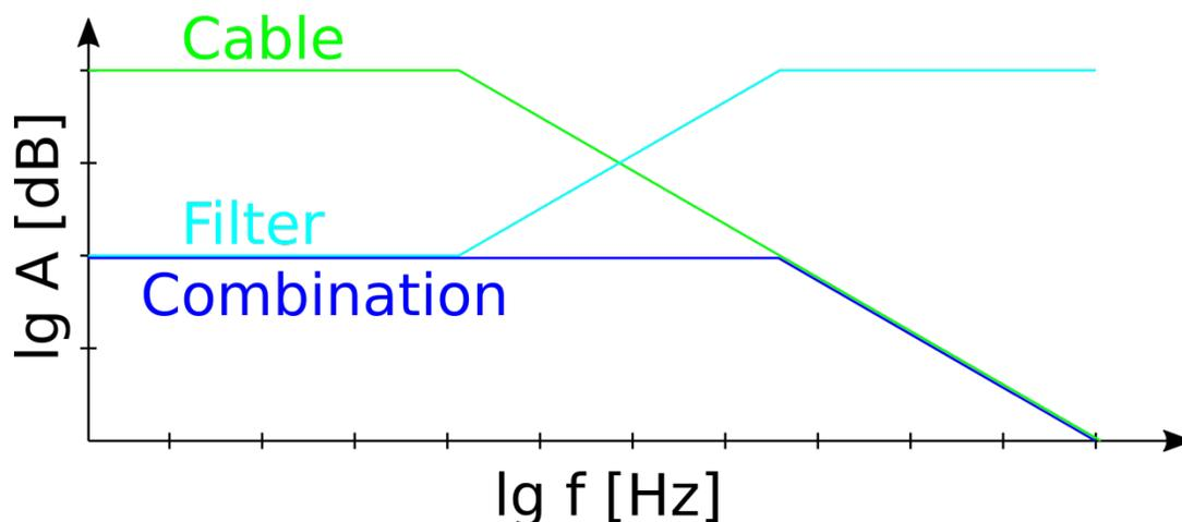
**Figure 5. Bode plot cable (green), filter (cyan) and the resulting overall transfer function (blue)**
