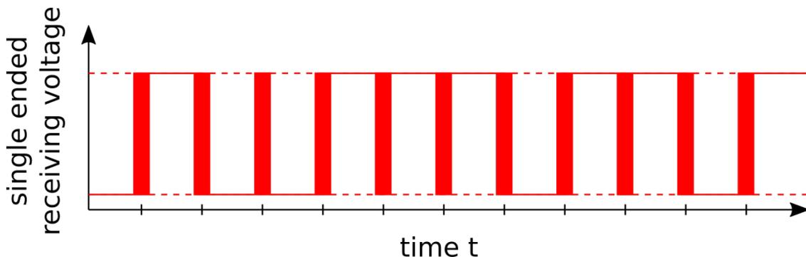
**Figure 4. Theoretical eye diagram of the output signal**
