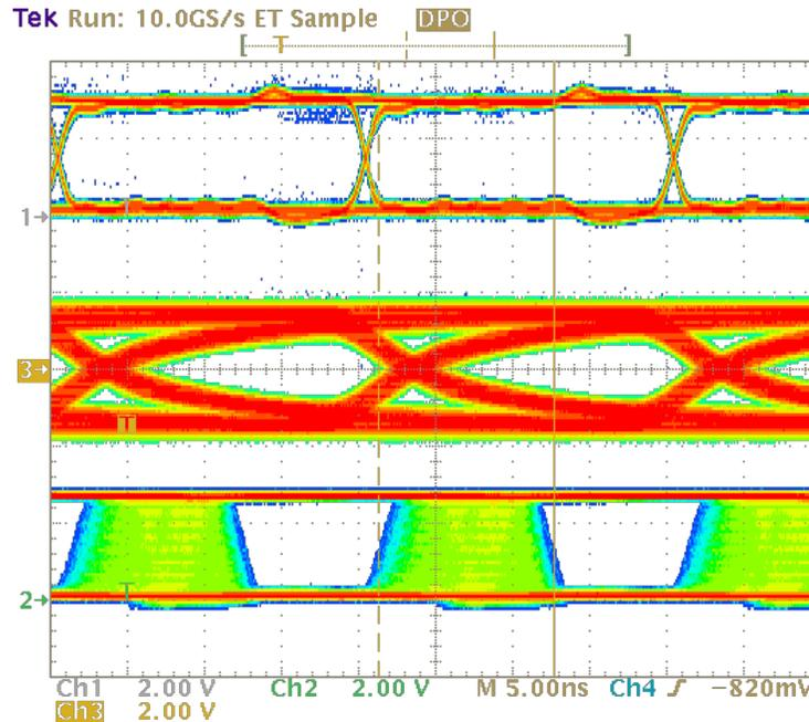
**Figure 9. 120Ω reference termination resistor on a 100m cable at 50Mbps and 11.4ns jitter. Differential channel resolution is 2V/div.**
