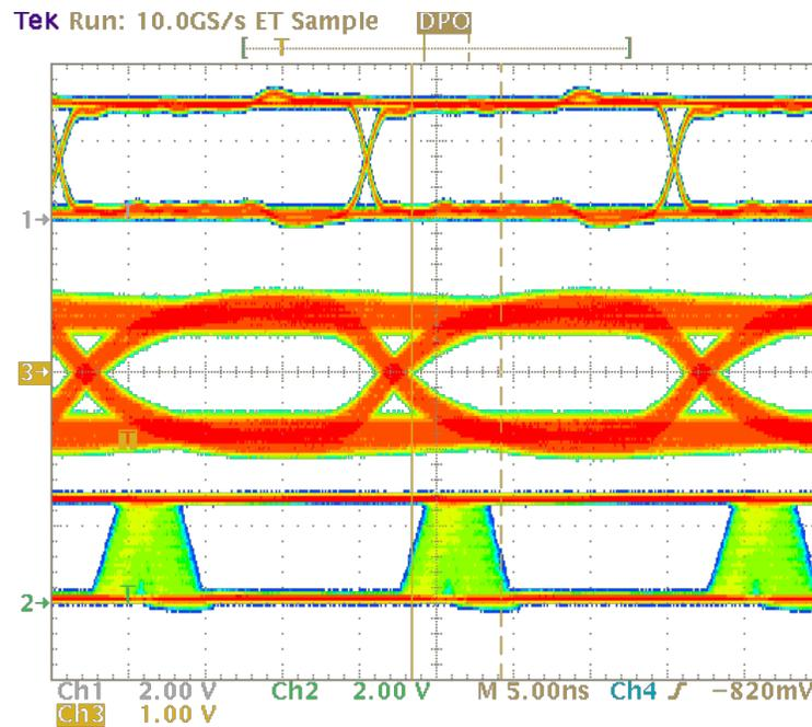
Figure 10. Passive equalizer eye diagrams on a 100m cable at 50Mbps and 5.8ns jitter. Parallel termination resistor 120Ω, series termination resistor 60Ω, series capacitor 680pF. Differential channel resolution is 1V/div.
