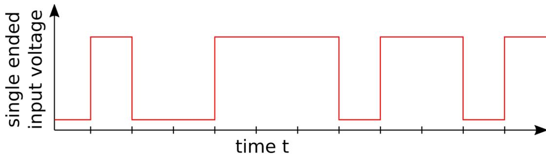
**Figure 2. Single ended input signal from UART**
