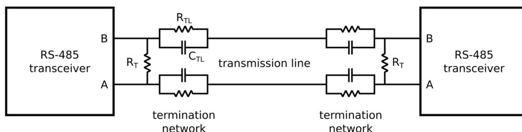
**Figure 6. Passive RS-485 equalizer circuit**
