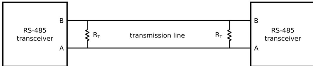
**Figure 1. Typical point to point RS-485 connection**
