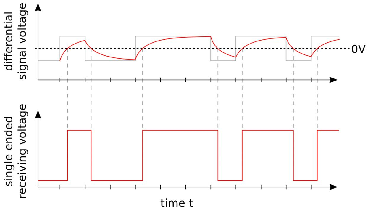
**Figure 7. Top: Theoretical (gray) and real (red) differential signal with the passive RS-485 equalizer**
