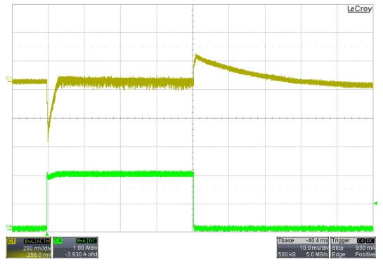
8.2 5mA to 2A Transient; 230VAC/50Hz Input
