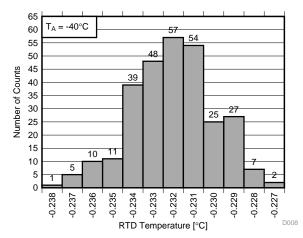
Figure 21. RTD Channel Histogram (280 Data Points) for PT100 =  $100 \Omega$  at  $-40^{\circ}$ C
