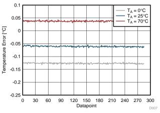
Figure 20. RTD Channel Temperature Error for PT100 = 100 Ω at 0°C, 25°C, and 70°C
