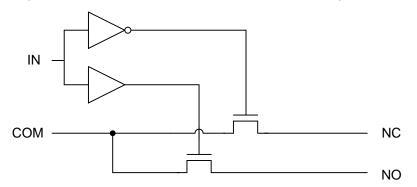
Figure 3. TS5A3159 Block Diagram
