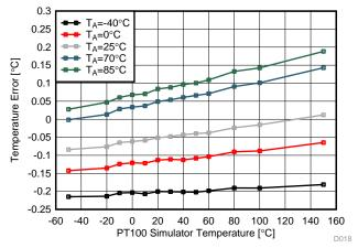
Figure 26. RTD Channel Temperature Error for Different PT100 Simulator Settings Across Ambient Temperature
