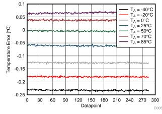
Figure 18. RTD Channel Temperature Error for PT100 = 100 Ω Across Ambient Temperature
