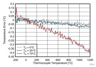
Figure 12. Thermocouple Temperature Error ( $T_A = 0^{\circ}C$  to 70°C)
