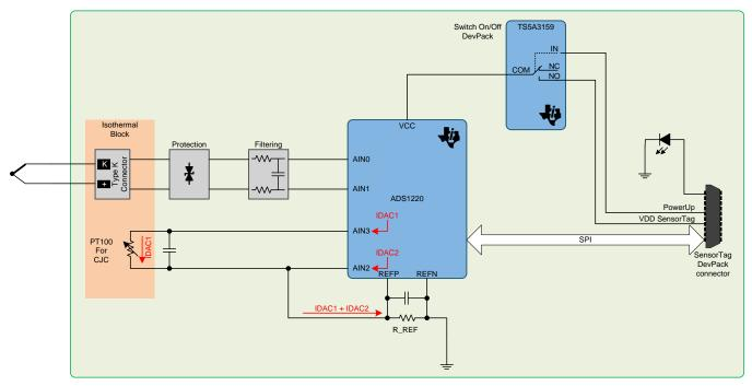
Figure 1. TIDA-00650 Block Diagram
