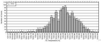
Figure 16. Thermocouple  $V_{IN} = 50 \text{ mV}$  at  $T_A = 70^{\circ}\text{C}$ ; Min/Max = 0.962
