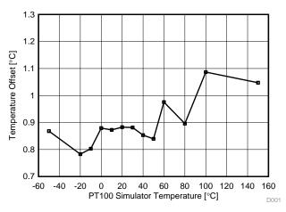
Figure 9. PT100 Simulator Equivalent Temperature Offset Including Test Wire
