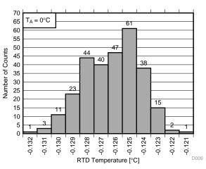
Figure 22. RTD Channel Histogram (280 Data Points) for PT100 = 100  $\Omega$  at 0°C
