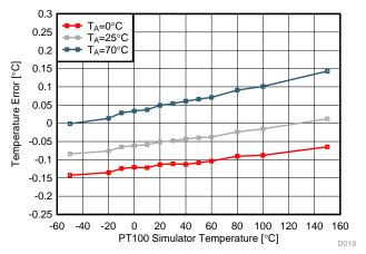
Figure 27. RTD Channel Temperature Error for Different PT100 Simulator Settings at 0°C, 25°C, and 70°C
