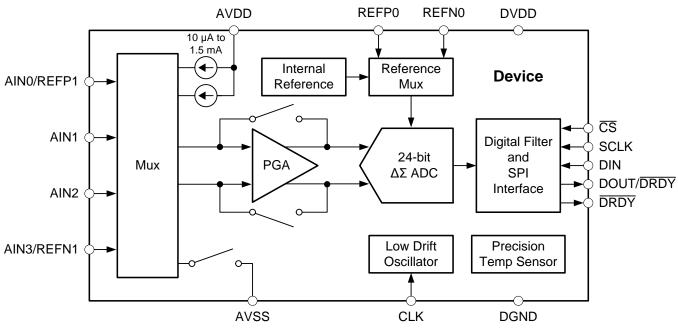
Figure 2. ADS1220 Functional Block Diagram
