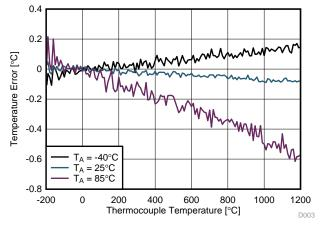
Figure 11. Thermocouple Temperature Error ( $T_A = -40^{\circ}C$  to 85°C)
