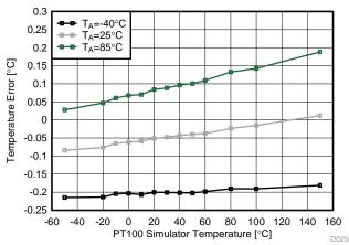
Figure 28. RTD Channel Temperature Error for Different PT100 Simulator Settings at -40°C, 25°C, and 85°C
