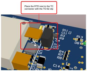
Figure 30. CJC Layout Requirements
