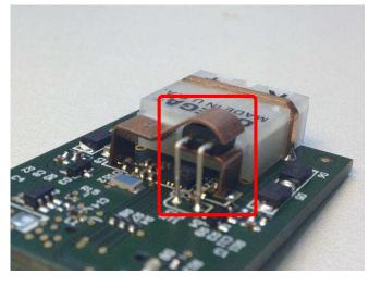
Figure 31. Assembly of PT100 on TC Connector Clip
