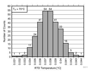
Figure 24. RTD Channel Histogram (280 Data Points) for PT100 =  $100 \Omega$  at  $70^{\circ}$ C
