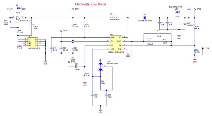
Figure 18. Boost Converter Schematic
