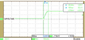
Figure 12. Capacitor Charging at  $V_{IN}$  = 30 V, 10-W Load
