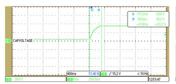
Figure 11. Capacitor Charging at  $V_{IN}$  = 24 V, 10-W Load
