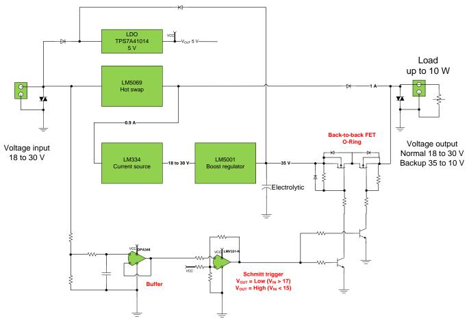
Figure 2. TIDA-00500 Block Diagram
