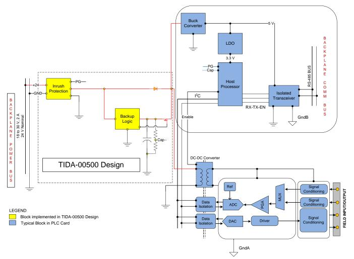
Figure 1. Generic Illustration of Power Block
