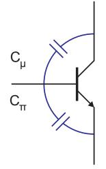
Figure 7. Internal Capacitance of BJT
