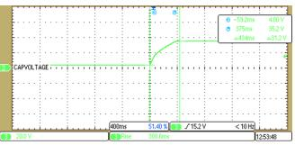
Figure 10. Capacitor Charging at  $V_{IN}$  = 18 V, 10-W Load
