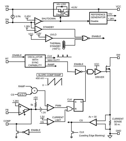
Figure 3. LM5001 Circuit Diagram
