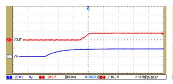
Figure 9. Startup at V<sub>IN</sub> = 18 V, 10-W Load
