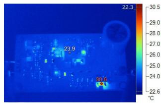
Figure 15. Thermal Analysis, Charging Mode With 10-W Load at  $V_{IN} = 18 V$
