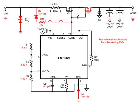
Figure 4. LM5069 With Reverse Polarity Protection
