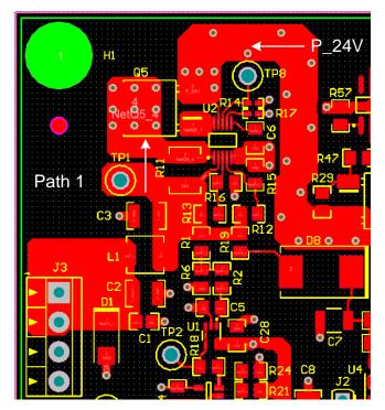
Figure 19. LM5069 Inrush Placement
