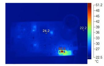
Figure 16. Thermal Analysis, Light Charging Mode With 10-W Load at  $V_{IN}$  = 18 V
